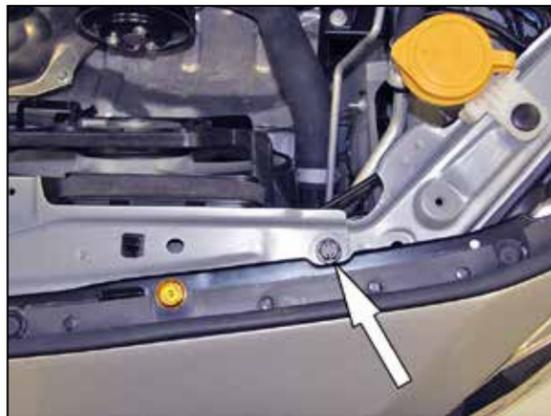
16. Remove the core support bolt shown.
