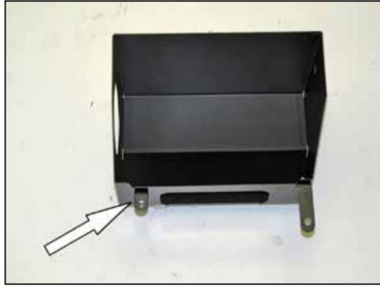
12. Install the provided "L" bracket (070066) onto the heat shield using the provided hardware.
