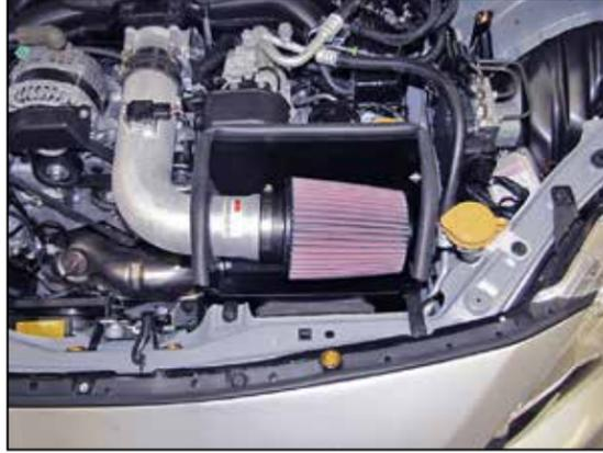
25. Install the K&N® air filter onto the K&N® intake tube and secure with the provided hose clamp. **NOTE: Drycharger® air filter wrap; part # RC-4630DK is available to purchase separately. To learn more about Drycharger® filter wraps or look up color availability please visit <http://www.knfilters.com>®.**
