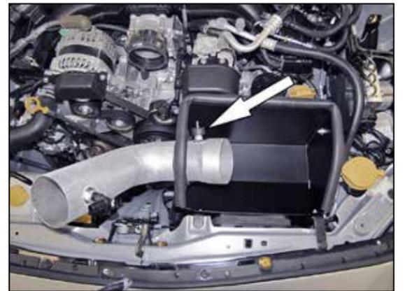
21. Install the tube through the heat shield and then install the provided rubber mounted stud onto the tube as shown.
