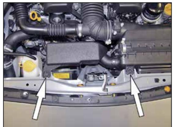
6. Remove the two bolts shown securing the resonator and air box to the core support.
