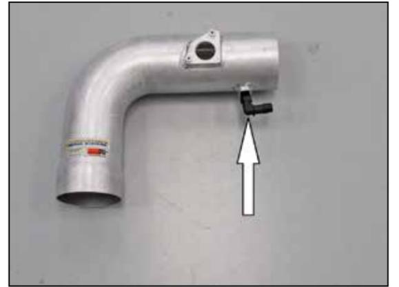
18. Install the provided 90° vent fitting into the K&N® intake tube as shown.
