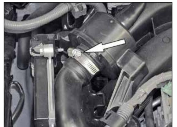
5. Loosen the hose clamp and disconnect the engine sound tube from the engine sound drum.
