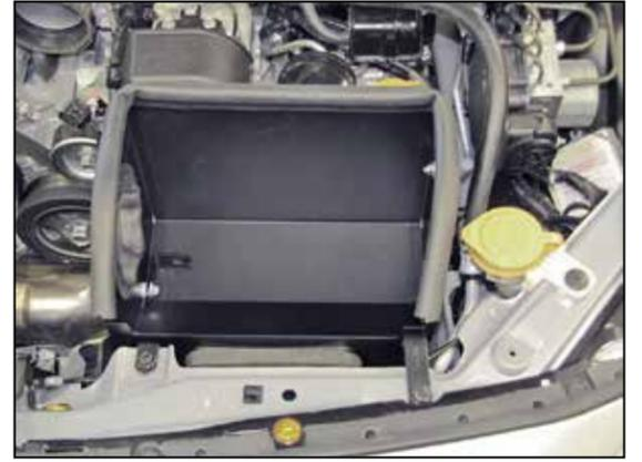
17. Set the heat shield into position on the core support and secure with the factory air box mounting bolts and to the previously install bracket with the hardware provided.
