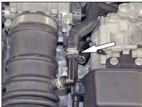
3. Release the spring clamp and then disconnect the crank case vent hose from the fitting.
