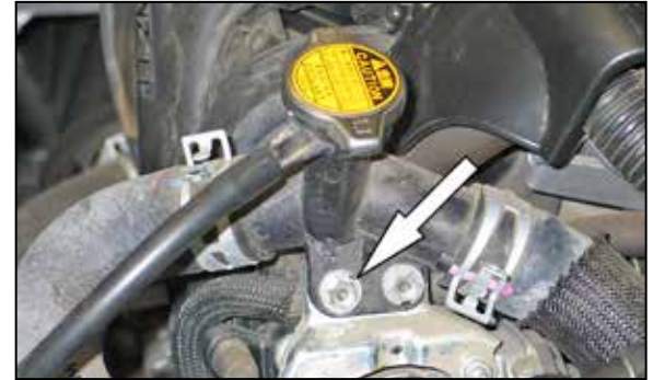
23. Remove the bolt securing the radiator fill neck to the radiator fill neck support (as shown).
