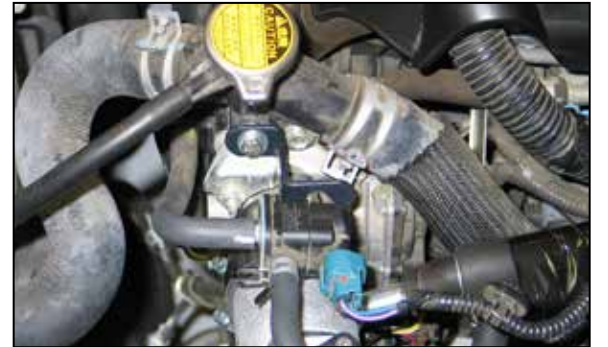
24. Install the vacuum switching valve assembly onto the radiator fill neck support with the provided hardware as shown.
