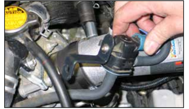
22. Install bracket (#07958) onto the vacuum switching valve with the provided hardware as shown.
