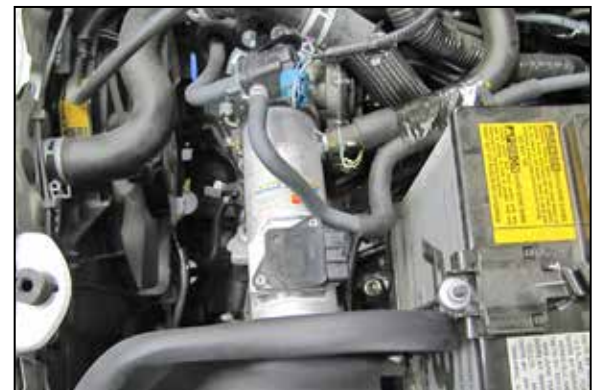
25. Install the crank case vent line onto the K&N® intake tube using the spring clamp removed in step # 4 (as shown).
