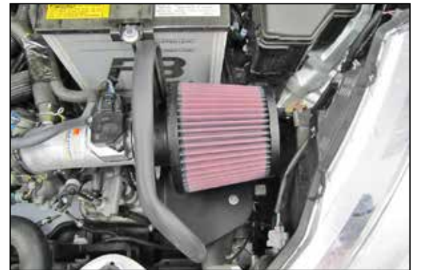
27. Install the K&N® air filter as shown. NOTE: Drycharger® air filter wrap; part # RX-4990DK is available to purchase separately. To learn more about Drycharger® filter wraps or look up color availability please visit http://www.knfilters.com .
