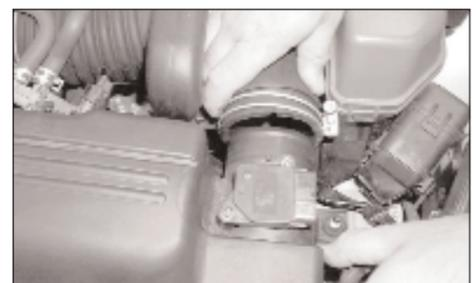
10. Remove the stock intake tube from the air cleaner assembly as shown.
