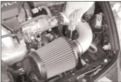
39. Install the K&N® air filter onto the intake tube as shown. Position the tube for best fit and clearance, then tighten all bolts and hose clamps.
