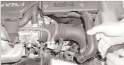
13. Remove the computer fresh air supply tube as shown.
