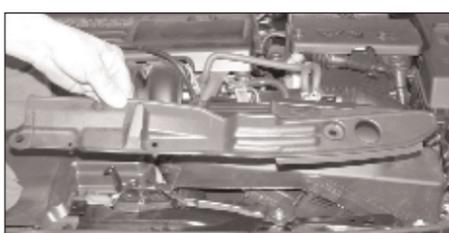
4. Remove the radiator core support cover as shown.
