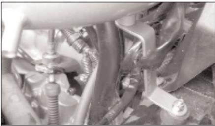
34. Secure the "Z" bracket to the threaded boss on the tube with the provided hardware.
