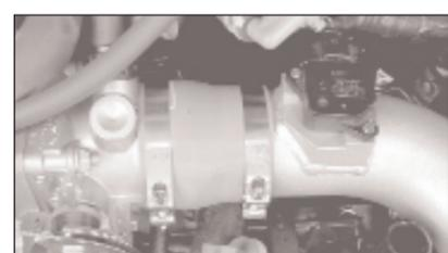
33. Install the intake tube onto the throttle body as shown but do not completely tighten the hose clamps at this time.
