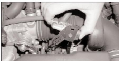
6. Unclip the PWM vacuum switching valve from the air cleaner assembly as shown.
