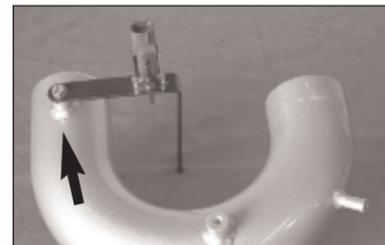
29. Install the "L" bracket onto the intake tube using the provided hardware as shown.
