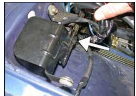
11. Unclip the wire harness from the bracket as shown.
