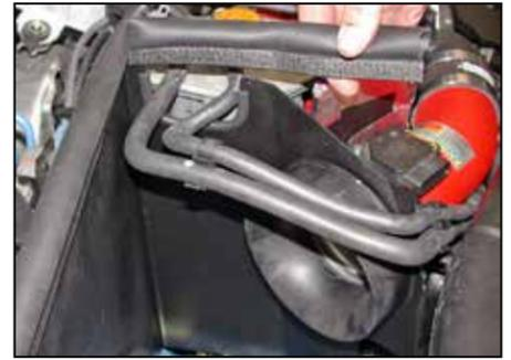
28. Install the remaining trim seal onto the heat shield and trim to fit as shown.
