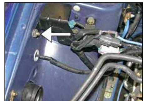
10. Remove the bolt on the wire harness bracket on the inner fender as shown.
