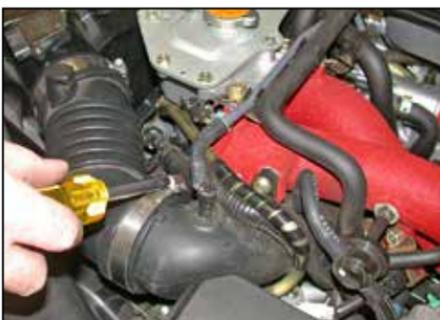
4. Loosen the hose clamp as shown.
