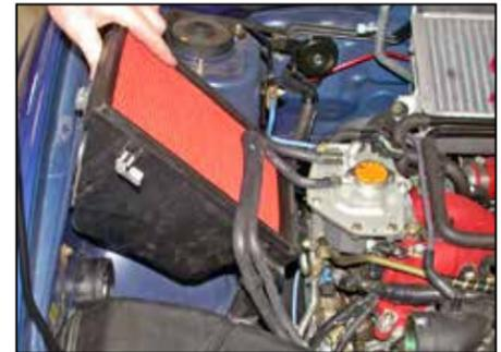
9. Remove the lower air cleaner assembly as shown.
