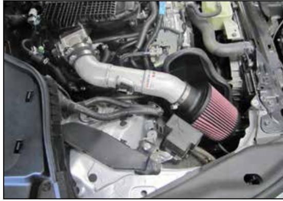
26. Install the K&N® air filter and secure with the provided hose clamp. Adjust the intake tube, heat shield and filter for pest fit and then secure all of the mounting points.
