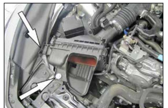
5. Remove the two bolts that secure passenger side air box and loosen the hose clamp to the intake tube.
