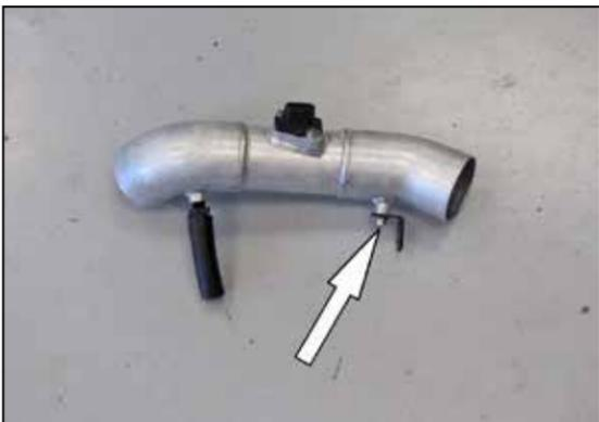
24. Install the tube mounting bracket (070066) onto the passenger side K&N® intake tube as shown but do not completely tighten at this time.
