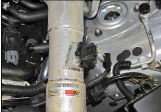
41. Reconnect the mass air sensor electrical connection.
