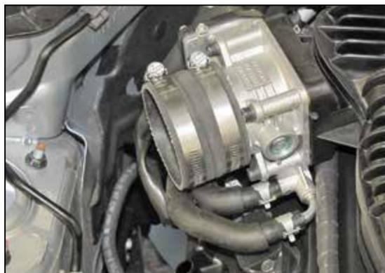
14. Install the provided coupling hose (08440) onto the passenger side throttle body and secure with the provided hose clamp.
