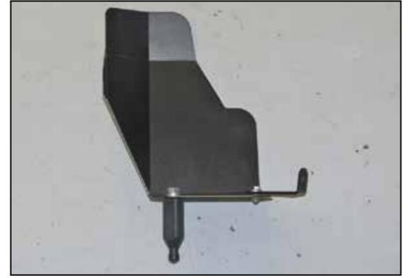
16. Install the provided mounting stud onto the passenger side heat shield and secure with the provided hardware.
