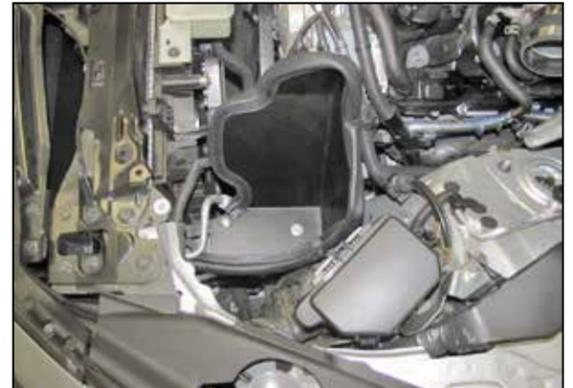
32. Install the heat shield into position as shown on the driver side frame rail and then secure to the core support with the provided hardware.
