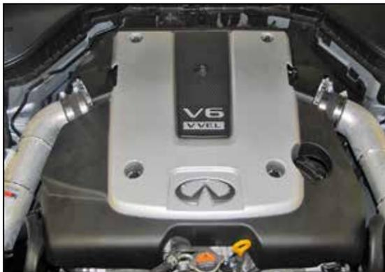
43. Reinstall the decorative engine cover and secure with the factory hardware.
