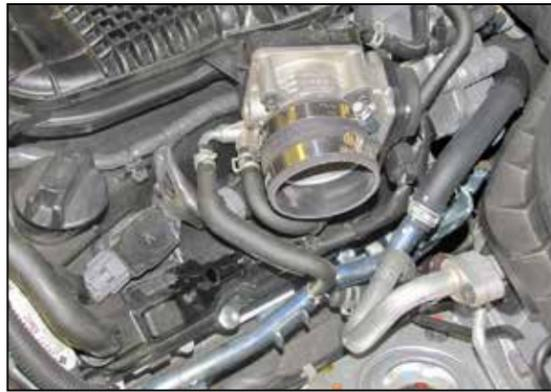
28. Install the remaining coupling hose (08440) onto the driver's side throttle body and secure with the provided hose clamp.
