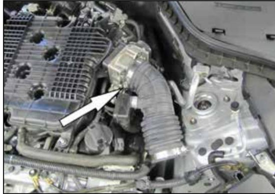
12. Loosen the hose clamp securing the driver's side intake hose to the throttle body.
