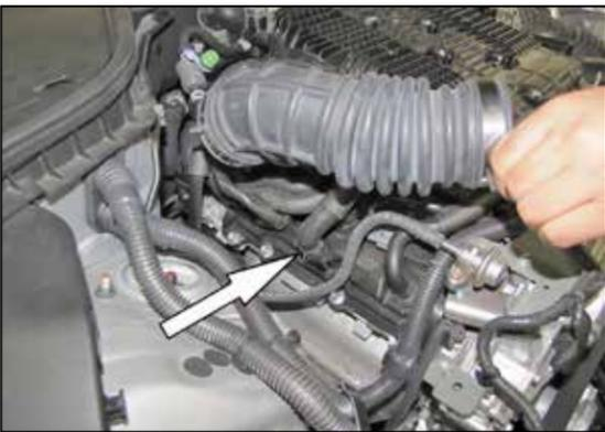
8. Pull the intake hose up to gain access to the crank case vent to valve cover connection. Release the clamp securing the crank case vent and then remove the passenger intake hose assembly.
