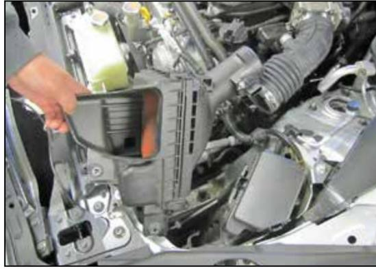
11. Remove the driver's side air box from the vehicle.
