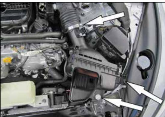
10. Remove the two bolts that secure driver side air box and loosen the hose clamp to the intake tube. **NOTE: The outer bolt is under a decorative cover, the cover will flex up enough to gain access to the bolt.**
