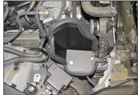
18. Install the heat shield into position as shown on the passenger side frame rail and then secure to the core support with the provided hardware. **NOTE: The mounting stud will insert into the factory air box mounting grommet.**
