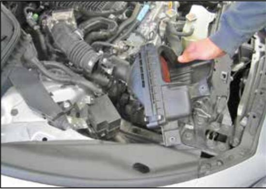
6. Lift up and remove the passenger side air box from the vehicle.
