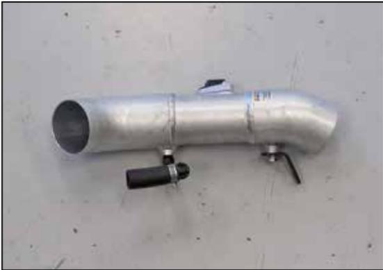
38. Install the tube mounting bracket (070049) onto the K&N® intake tube and secure with the provided hardware.
