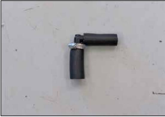
36. Install the 5/8" and 1/2" crank case vent hose's onto the 1/2" 90° fitting.
