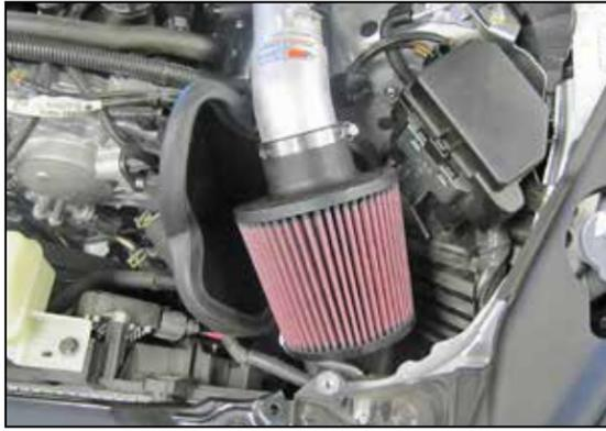
40. Install the K&N® air filter and secure with the provided hose clamp. Adjust the intake tube, heat shield and filter for pest fit and then secure all of the mounting points.
