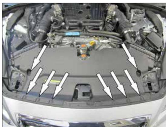
3. Release the eight clips securing the core support decorative cover and then remove the cover from the vehicle.
