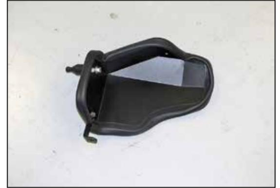
17. Install one of the provided edge trim pieces onto the passenger side heat shield as shown. **NOTE: It will be necessary to trim the edge trim for proper fit.**
