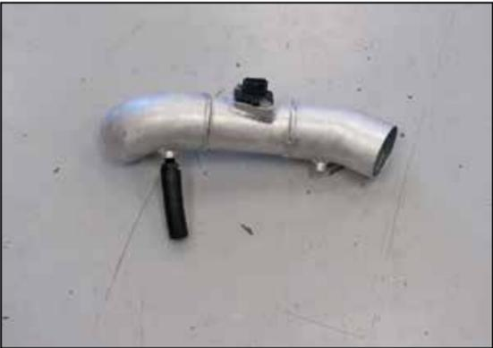
23. Install the 3-1/4" long section onto the fitting installed into the passenger side K&N® intake tube as shown.
