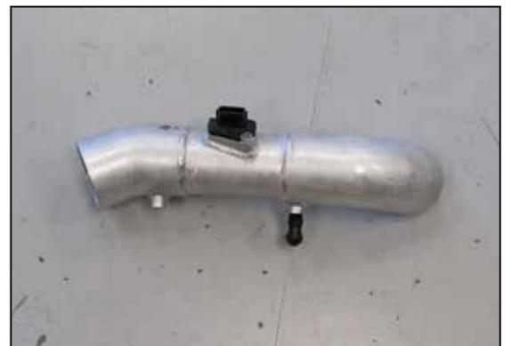
35. Install the mass air sensor into the K&N® intake tube and secure with the provided hardware.
