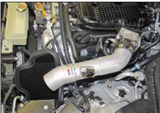
39. Install the driver side K&N® intake tube assembly into the coupling hose at the throttle body and the crank case vent hose onto the valve cover port. Align the mounting bracket with the hole in the heat shield and secure with the provided hardware. Do not completely tighten the mounting points at this time.
