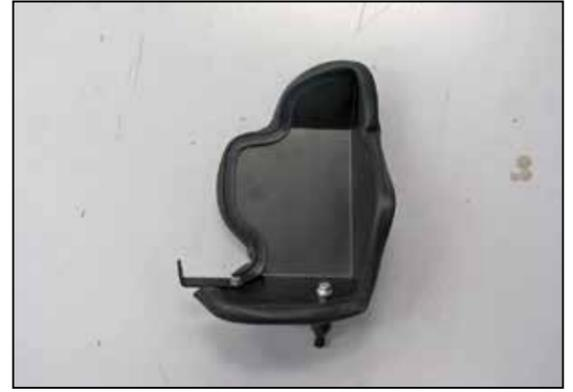
31. Install one of the provided edge trim pieces onto the driver's side heat shield as shown.
