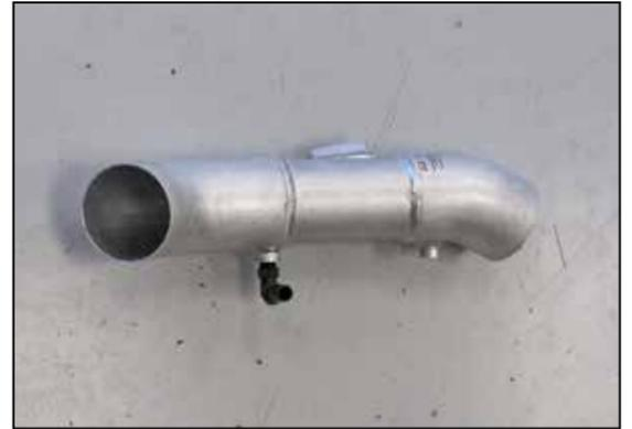
33. Install the provided 90° vent fitting into the passenger side K&N® intake tube (27620) as shown.
