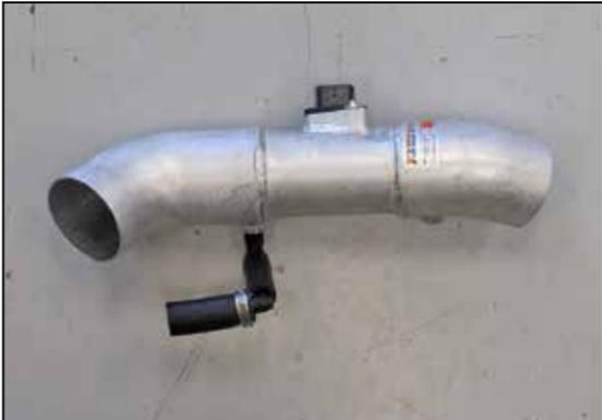
37. Install the vent assembly onto the vent fitting installed into the K&N® intake tube.
