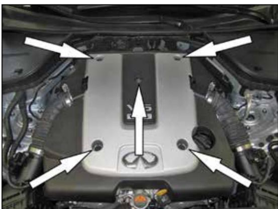
2. Remove the three bolts and two nuts securing the decorative engine cover and then remove the engine cover.
