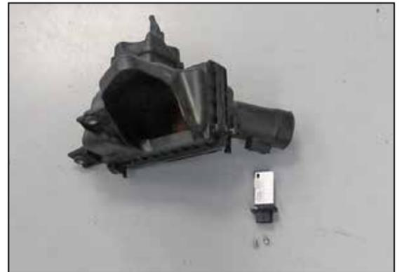
34. Remove the two screws securing the driver's side mass air sensor into the air box and then remove the sensor.
