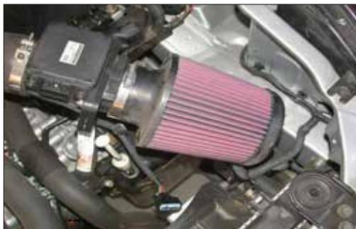
19. Install the K&N® air filter onto the mass air adapter and secure with the provided hose clamp
