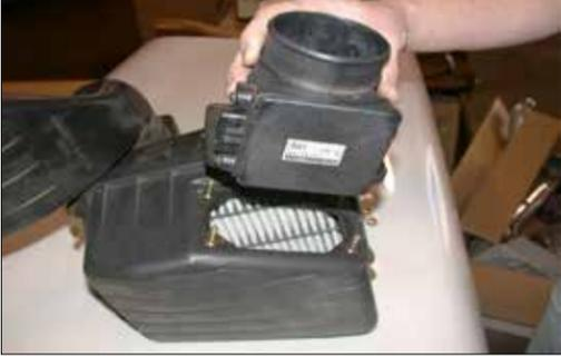
11. Remove the four nuts that secure the mass air sensor, then, remove the mass air sensor as shown.
