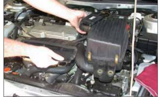
7. Loosen and remove the three bolts that secure the air cleaner assembly, then, remove the air cleaner assembly as shown.
