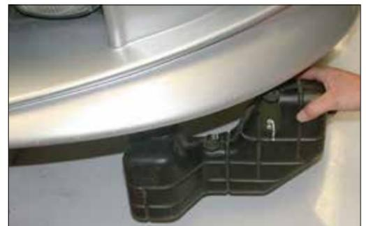
9. From underneath the vehicle remove the lower valance and loosen the three bolts that secure the air intake resonator to the inner fender, then, remove the air intake resonator from underneath the vehicle as shown.
