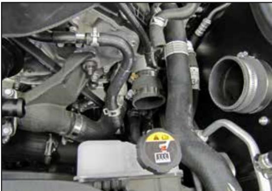
14. Install coupling hose (08638) onto the turbo inlet and secure with the provided hose clamp.
