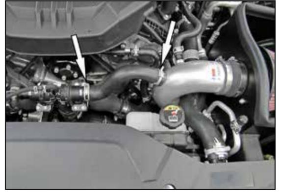
17. Install the passenger side BOV hose onto the driver side intake tube and BOV valve, secure with the factory spring clamps. Connect the vent lines to the fittings installed into the K&N® intake tube.
