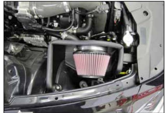
21. Install the passenger side heat shield assembly into the vehicle so the fresh air intake inserts into the opening of the heat shield and then secure the heat shield with the provided hardware.
