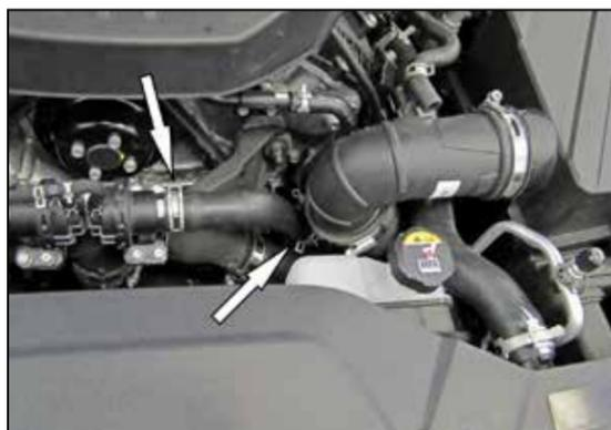
4. Release the spring clamps that secure the driver side BOV hose to the BOV and intake tube, then remove the driver side BOV hose.
