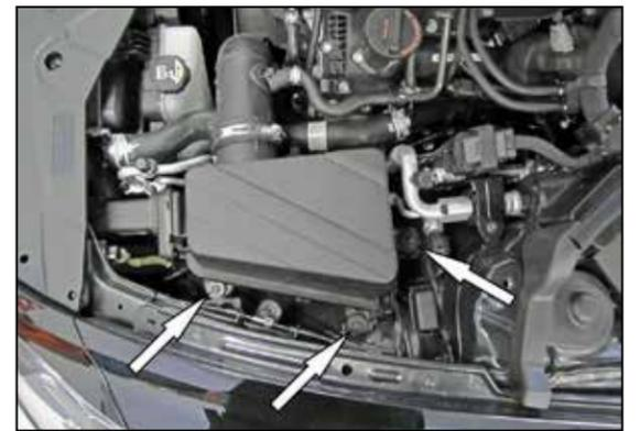
5. Remove the three bolts that secure the driver side air filter housing to the inner fender, loosen the hose clamp that secures the intake tube to the air filter housing and disconnect the tube. Remove the driver side air filter housing from the vehicle.
