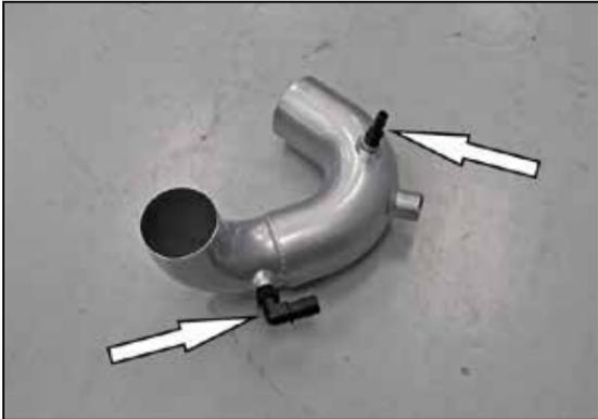
15. Install the NPT vent fittings into the driver side K&N® intake (27677) as shown.
