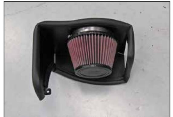
20. Install the remaining air filter onto the passenger side filter adapter as shown and secure with the provided hose clamp.
