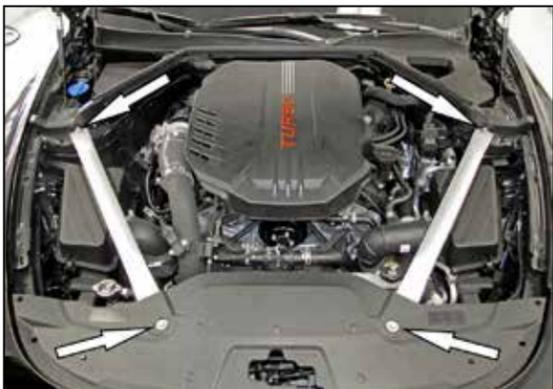
2. Remove the four bolts shown that secure the two strut tower braces to the vehicle and then remove the braces from the vehicle.
