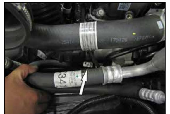
6. Loosen the hose clamp that secures the intake tube to the driver side turbo and then remove the intake tube from the vehicle.
