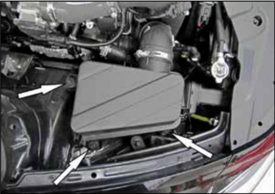
8. Remove the three bolts that secure the passenger side air filter housing to the inner fender, loosen the hose clamp that secures the intake tube to the air filter housing and disconnect the tube. Remove the passenger side air filter housing from the vehicle.
