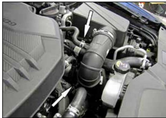
3. Release the spring clamps that secure the two vent lines attached to the driver's side intake tube and then disconnect the vent lines from the intake tube.
