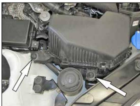
4. Remove the two bolts which secure the factory air box to the inner fender.
