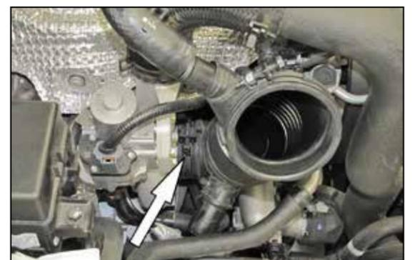
6. Loosen the hose clamp securing the factory intake hose to the turbo inlet. Remove the factory intake hose from the vehicle.
