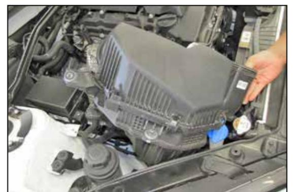
5. Disconnect the factory intake hose and then remove the complete air box assembly from the vehicle.
