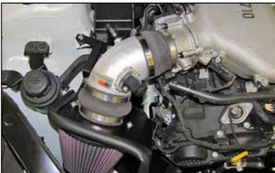
27. Install the K&N® intake tube all the way into the hump hose and then align with the throttle body. Install the step hose onto the throttle body and adjust the tube and hoses for best fit. Then secure the tube and hoses with the provided hose clamps.
