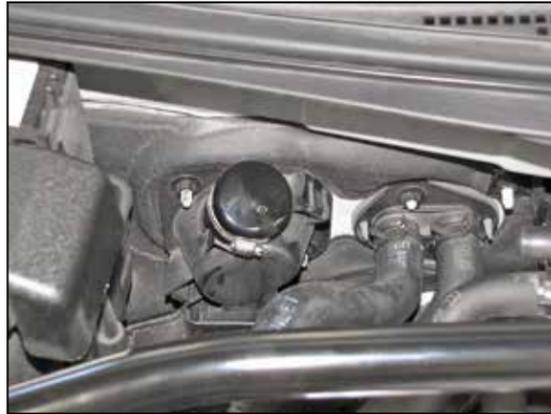
13. Install the provided cap onto the fitting in the fire wall for the sound drum.
