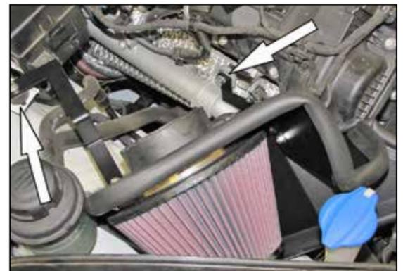
20. Set the filter assembly into position and secure to the rubber mount and coolant tube mounting location with the provided hardware.
