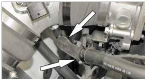
31. Install the 4.5" breather hose onto the 90° fitting in the K&N® intake tube and then attach the hose mender into the crank case breather hose as shown.
