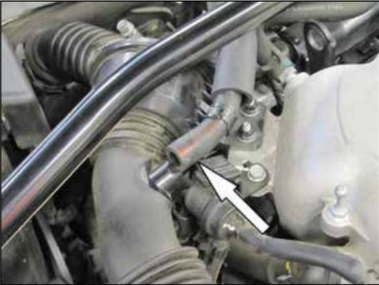
9. Disconnect the vent line from the engine sound tube.
