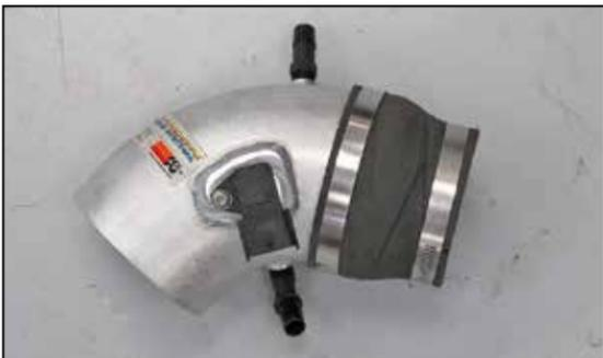
26. Install the step hose (08497) onto the K&N® intake tube as shown. Do not tighten the hose clamp at this time.
