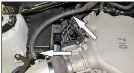
30. On vehicles equipped with a vent hose attached to the sound tube, install the 11" breather hose onto the fitting in the intake tube and then attach the hose mender into the EVAP breather hose as shown.
