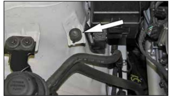
18. Install the provided rubber mounted stud onto the air box mounting location on the inner fender as shown.
