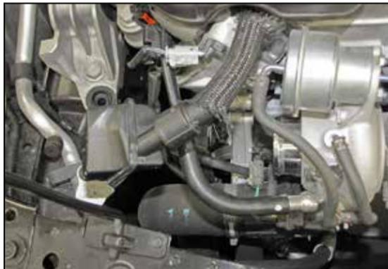
15. Reposition the crank case vent hose and chamber above the coolant by-pass hose.
