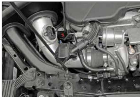
18. Install the crank case vent breather chamber into the hose installed onto the K&N® intake tube.
