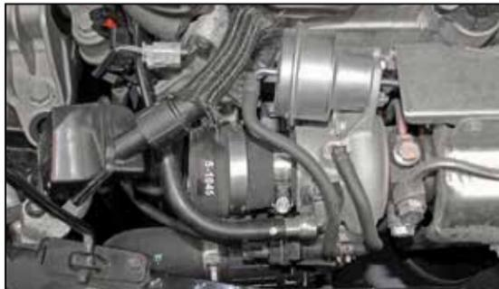
16. Install the provide coupler hose (5-1045) onto the turbo and secure with the provided hose clamp.
