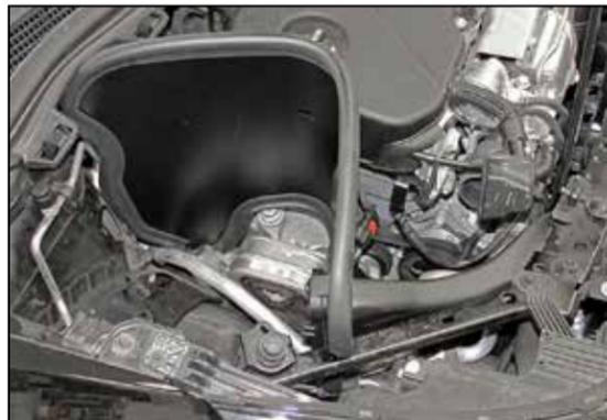
17. Install the heat shield so the fresh air intake goes into to its correct position and the mounting studs engage with the factory grommets. Reinstall the fresh air retaining pin remove in step #2.
