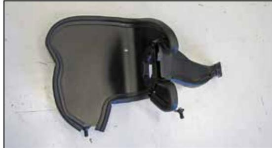
14. Install the factory fresh air duct into the heat shield as shown.
