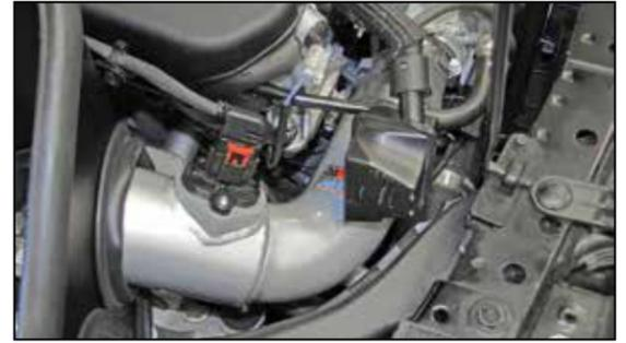
19. Reconnect the mass air sensor electrical connection.
