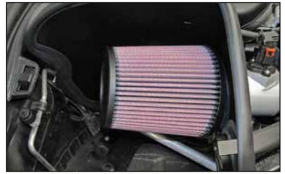
20. Install the K&N® filter and secure with the provided hose clamp.
