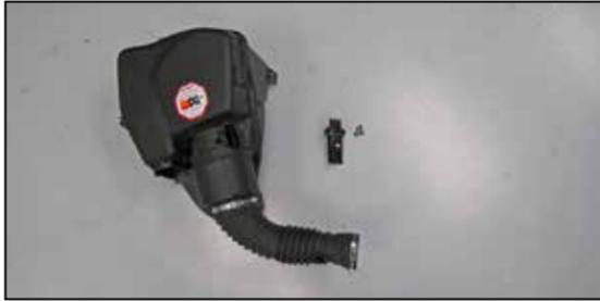
8. Remove the mass air sensor from the factory air filter housing.
