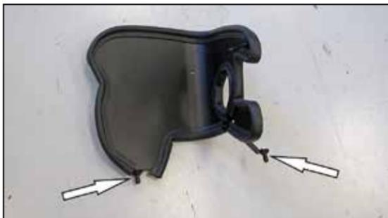
12. Install the two provided mounting studs onto the heat shield where shown.
