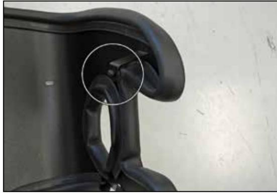
13. Install the rubber plug provided into the heat shield where shown.
