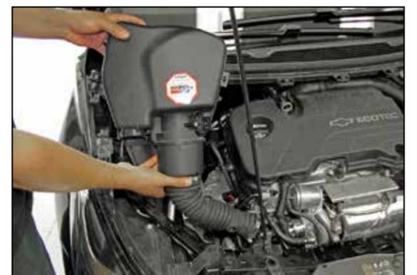
6. Lift up and remove the complete stock intake system from the vehicle.
