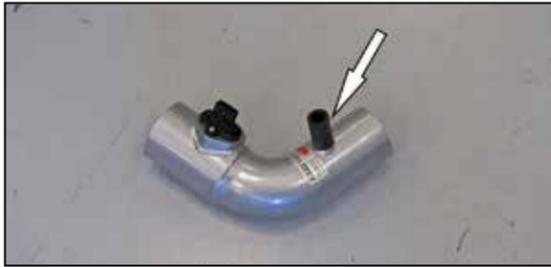
10. Install the provided crankcase vent hose onto the K&N® intake tube as shown.
