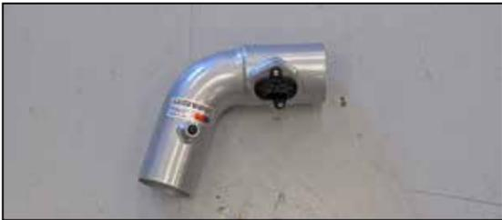
9. Install the mass air sensor into the K&N® intake tube and secure with the proper hardware.
