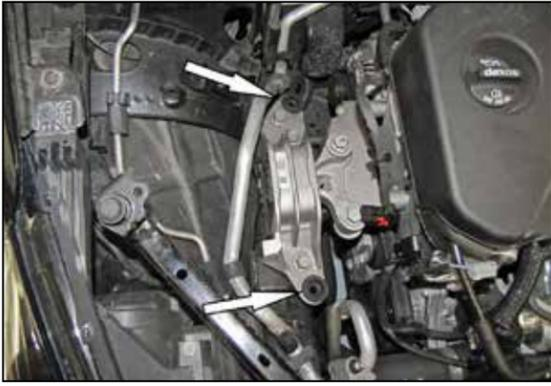
7. Be sure the factory air filter housing grommets are still in place on the mounts.
