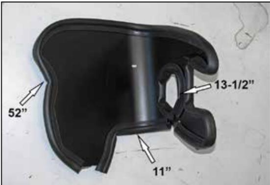
11. Cut the provided edge trim into three sections, one will be 52" long, one will be 13-1/2" long and the last one will be 11" long. Install the edge trim onto the heat shield as shown.
