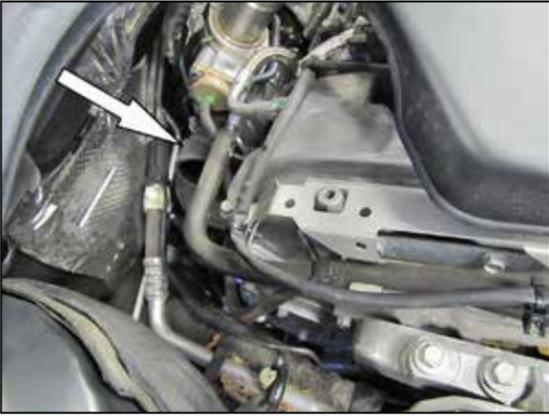
7. Install the provided coupling hose (084016) onto the turbo inlet and secure with the provided hose clamp.
