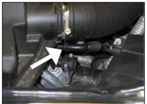
3. Disconnect the airbox drain tube from the airbox. **NOTE: The drain tube will pull straight out from the airbox.**
