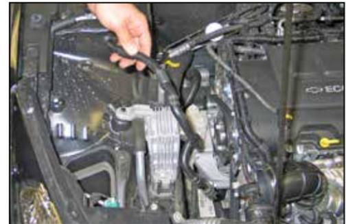
6. Unhook the two clips that secure the airbox drain tube to the inner fender, and then remove the drain tube from the vehicle.
