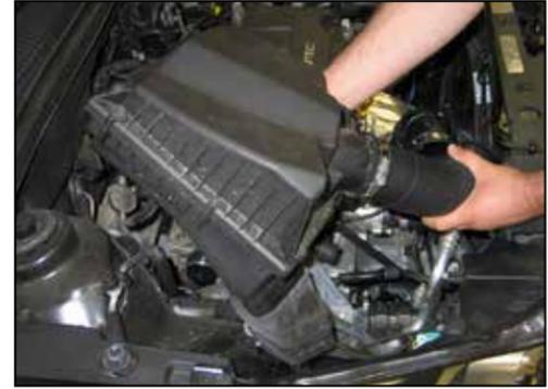
5. Lift the airbox assembly to dislodge it from the mounting grommets and then remove the airbox from the vehicle. **NOTE: K&N Engineering, Inc., recommends that customers do not discard factory air intake.**
