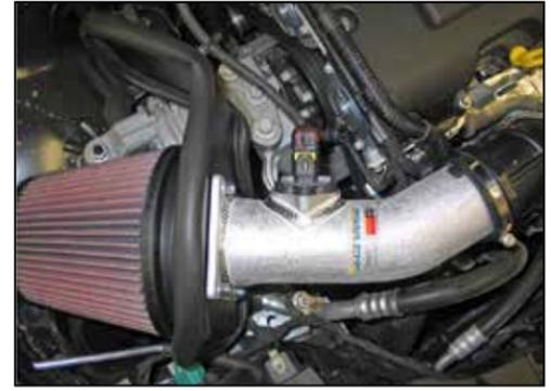
18. Connect the mass air sensor electrical connection.
