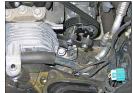
9. Install the heat shield mounting bracket onto the motor mount and secure with the factory bolt removed in step #7. **NOTE: Do not completely tighten at this time.**
