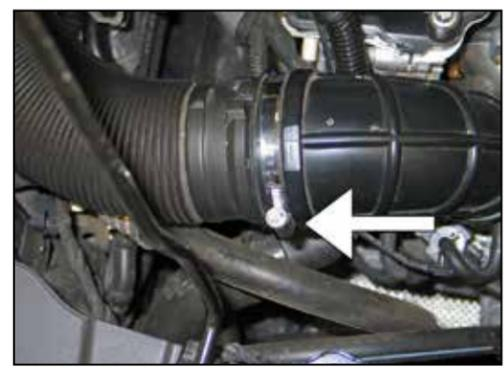
4. Loosen the hose clamp securing the stock intake tube to the intake elbow.
