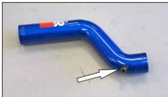
15. Install the grommet provided and the factory inlet air temperature sensor into the K&N® intake tube as shown.
