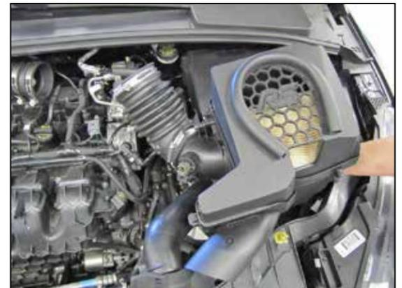
6. Lift and dislodge the air box from its mounting grommets and then remove the air box from the vehicle.
