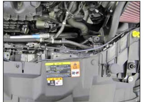
21. Using the K&N® Fresh air duct as a guide, mark the two hole locations onto the fresh air duct in the core support. Next remove the K&N® fresh air duct and drill two 1/4" id holes into the factory fresh air duct in the core support at the marked locations.
