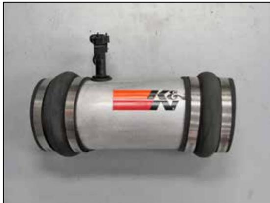
15. Install both of the coupling hoses (08418) onto the K&N® intake tube as shown.
