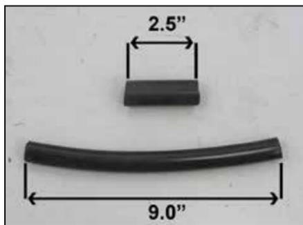
19. Cut the provided 1/2" silicone vent hose to a length of 9" long. Also cut the 5/8" vent line to a length of 2.5" long.
