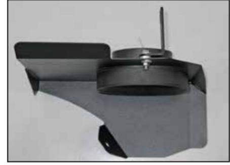
9. Install the provided heat shield mounting bracket (070742) along with the spacer onto the heat shield as shown.
