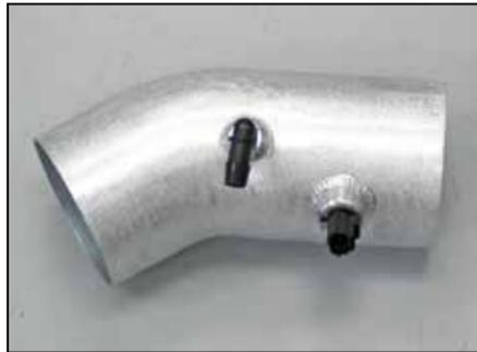
17. Install the inlet air temperature sensor into the K&N® intake tube as shown.
