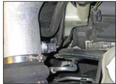
22. Reconnect the inlet air temperature sensor electrical connection.
