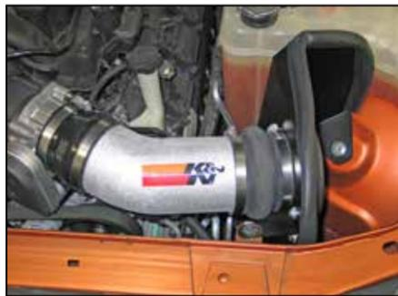
18. Install the K&N® intake tube into the silicone hump hose and then into the silicone step hose at the throttle body. Align the intake tube and heat shield for proper fit and then secure the intake tube with the provided hose clamps and heat shield bracket with the factory air box retaining bolt removed in an earlier step.
