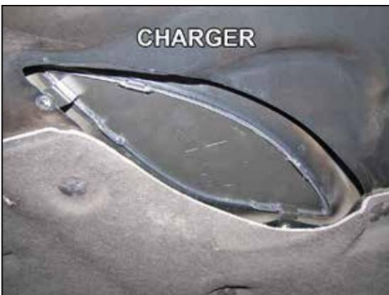
26. Install the guard so the mounting tabs are between the hood and the factory grid as shown.
