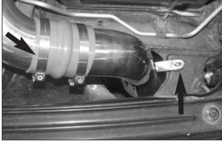
17. Install the K&N® Typhoon® cold air tube into the vehicle and line up the bracket with the rubber mounted stud, then, slide the silicone hose over the K&N Typhoon short ram tube as shown.
