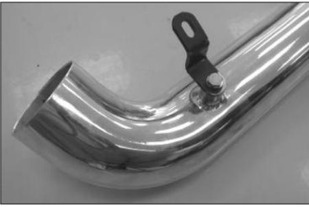
11. Using the provided hardware secure the provided "Z" bracket to the K&N® Typhoon® short ram tube as shown.
