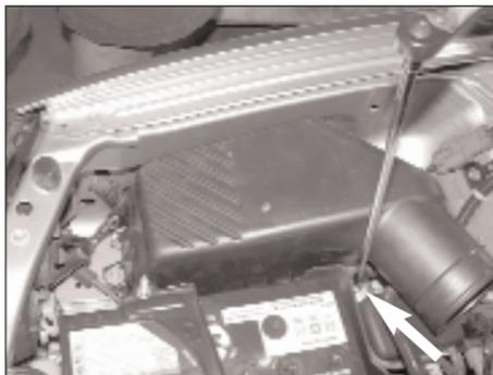
7. Loosen the two bolts that secure the air cleaner assembly as shown.
