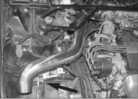
12. Slide the K&N® Typhoon® short ram tube into the silicone hose at the throttle body, then line up the bracket with the rubber mounted stud as shown.
