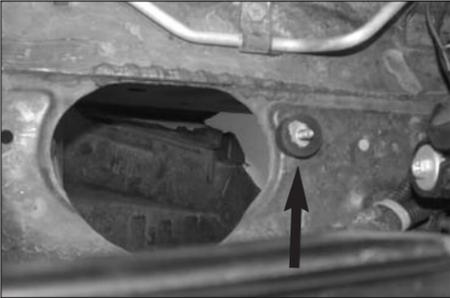
14. Install the rubber mounted stud into the air cleaner mounting hole as shown.
