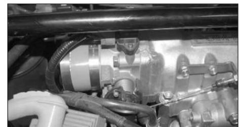
9. Install the silicone hose and hose clamps onto the throttle body as shown, using a flat blade screwdriver.
