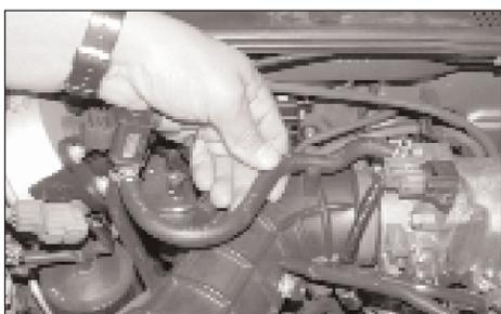
4. Remove the EVAP vent hose from the rubber clip on the intake tube as shown.
