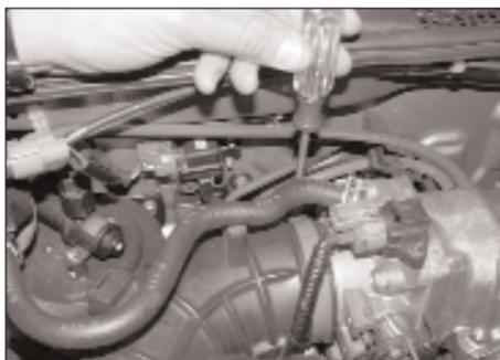
5. Loosen the hose clamp at the throttle body as shown.
