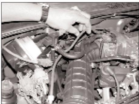
3. Remove the vacuum hose from the rubber clips on the stock intake tube as shown.
