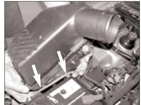
8. Pull upwards to remove the air cleaner assembly as shown.
