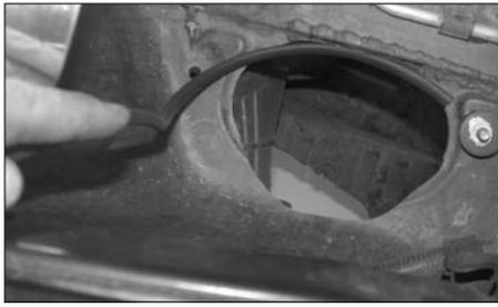
16. Install the provided edge trim into the hole in the inner fender as shown.
