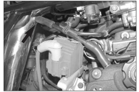
22. Slide the provided silicone hose onto the stock crank case vent hard line, then, secure the other end to the vent on the K&N® typhoon® short ram tube as shown.
