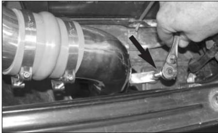
18. Using the provided hardware secure the bracket to the rubber mounted stud as shown.
