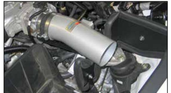
19. Install the K&N® intake tube into the silicone hose at the throttle body and align with the mounting bracket. Secure with the hose clamp and provided hardware.
