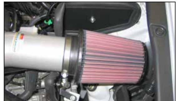
21. Install the K&N® air filter onto the intake tube and secure with the provided hose clamp.
