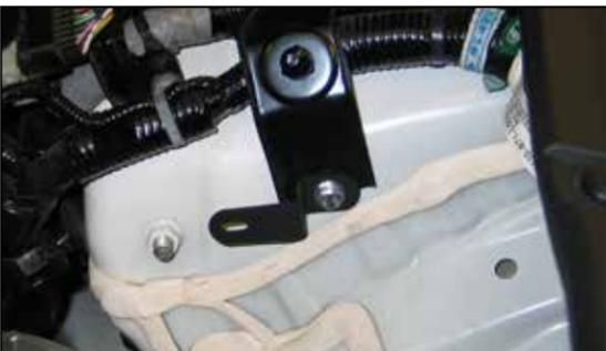
11. On Honda vehicles, install the heat shield mounting bracket (070116) onto the air box mounting bracket and secure with the provided hardware.
