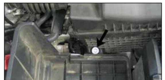
6. Loosen the bolt which secures the lower airbox to the battery tray.
