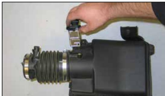
17. Remove the mass air sensor from the stock airbox.
