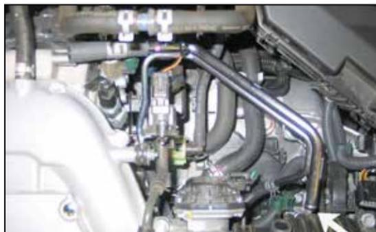
4. Disconnect the crankcase vent tube from the intake tube and valve cover port as shown. The spring clamps will not be reused.
