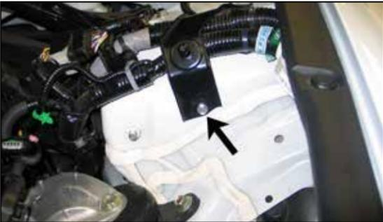
10. On Honda vehicles, remove the airbox mounting bracket bolt shown.
