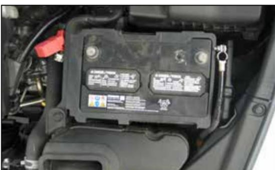
2. Disconnect the positive battery cable, remove the battery hold down and then remove the battery.
