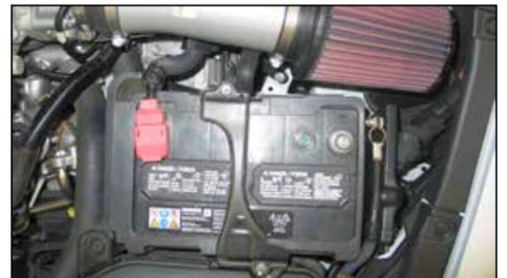
22. Reinstall the battery and secure with the hold down bracket. Reconnect the positive battery cable.
