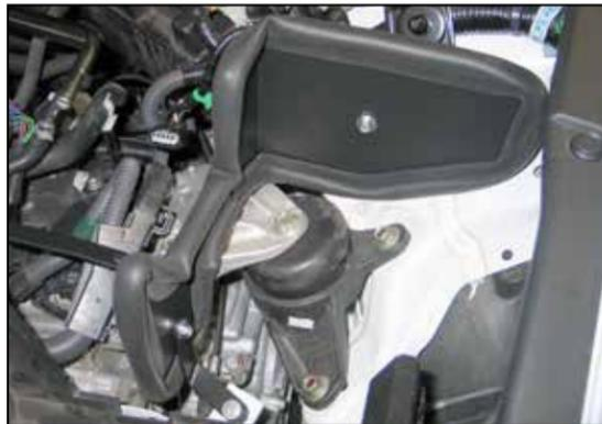
14. Install the heat shield assembly into the vehicle and secure to the mounting brackets with the hardware provided.
