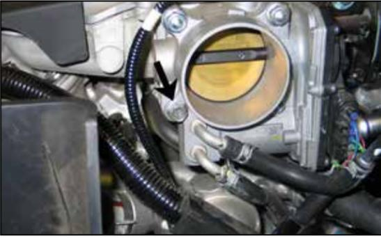
8. Remove the front lower throttle body bolt shown.
