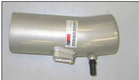
16. Install the 1/4" NPT fitting into the K&N® intake tube as shown.
