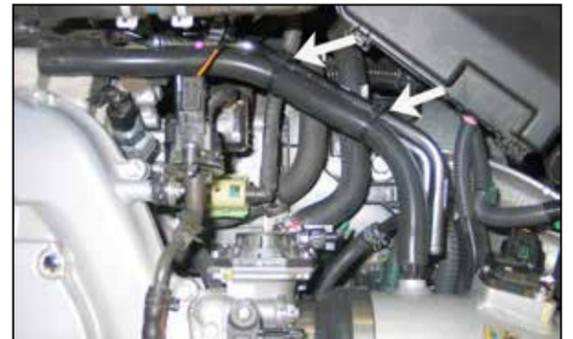
20. Install the provided crankcase vent hose onto the NPT fitting and then onto the valve cover port. Secure the crankcase hard line to the provided hose with the tie wraps provided.
