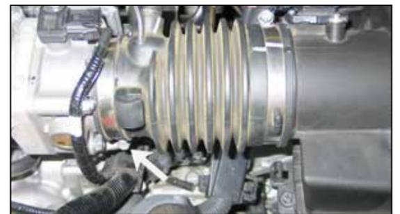
5. Loosen the hose clamp which secures the stock intake tube to the throttle body.
