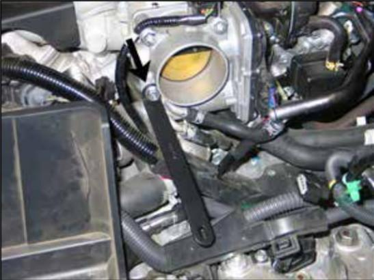
9. Install the tube mounting bracket (070114) onto the throttle body and secure with the bolt removed in the previous step.
