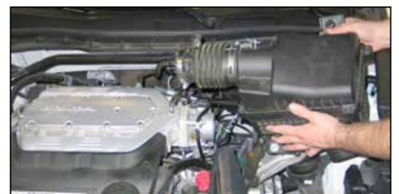
7. Remove the airbox assembly from the vehicle; be sure to unhook the wiring harness from the airbox as it is removed.
