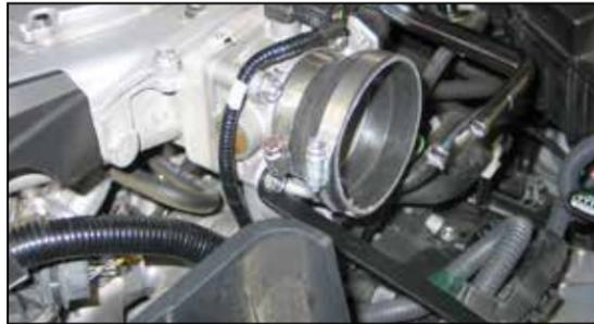
15. Install the silicone hose (084093) onto the throttle body and secure with the provided hose clamp.
