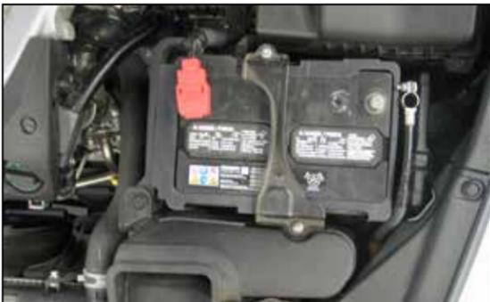
1. Turn off the ignition and disconnect the negative battery cable.
