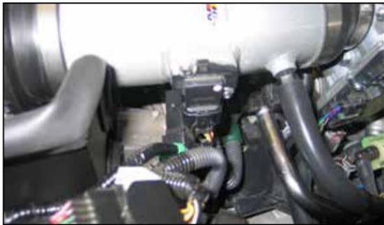
23. Reconnect the mass air sensor electrical connection.
