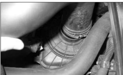
5. Unclip the intake tube and pull it from the air box lid as shown.
