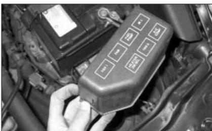
8. Remove the plastic cover from the relay box as shown.
