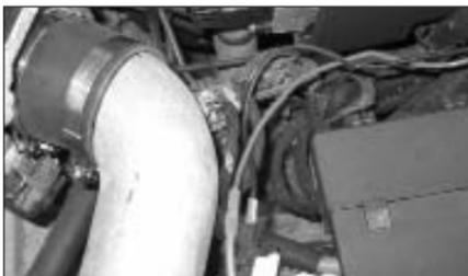
42. If necessary, reposition any cables away from the intake tube and secure them with a plastic cable tie supplied.
