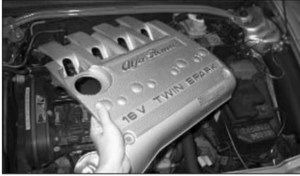
2. Remove the oil filler cap, undo the 4 fixing screws and remove the engine cover from the vehicle as shown.
