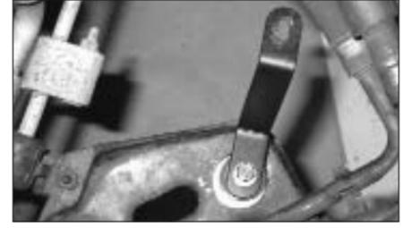
29. Fit the "Z" bracket to the rubber vibration mount as shown, using a Nylock nut and flat metal washer supplied. Don't fully tighten yet!
