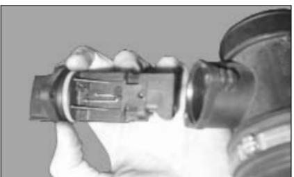
21. Using the provided Torx (69801) unscrew and carefully remove the MAS from its housing as shown.
