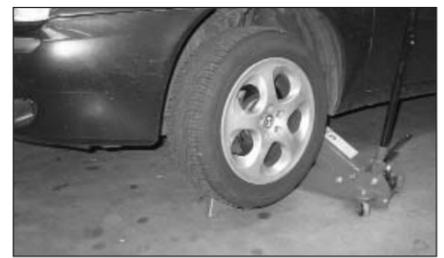
13. As per manufacturer's instructions and taking all necessary safety precautions, carefully raise the front of the vehicle and support it with a pair of axle stands.
