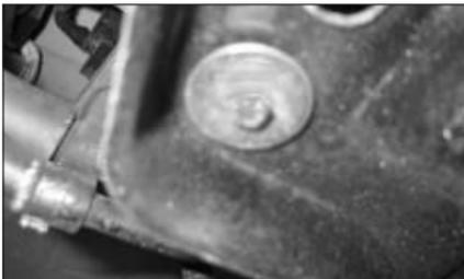
28. From underneath the vehicle, fit the assembly from step #27 to the rubber vibration mount over the air box mounting hole as shown. Don't fully tighten yet!
