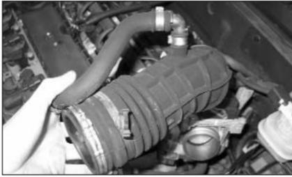
7. Undo the hose clamp at the throttle body, release the intake hose from and remove the intake hose from the vehicle as shown.
