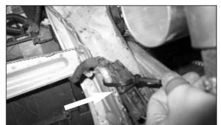
32. From underneath the vehicle, secure the indicated electrical connector to the hole in the chassis using a cable tie supplied as shown.
