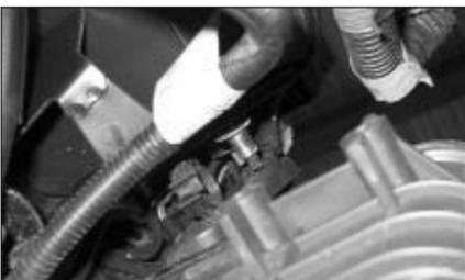
18. Unclip the cable harness from the air box and push the air box from its mounting stud as shown. Pull the air box from its rubber gromets and carefully remove it from the vehicle.
