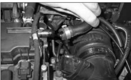
4. Unclip the breather hose from the vent on the engine as shown.
