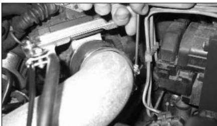
37. Adjust the intake tube for maximum clearance from the battery; now firmly tighten the hose clamp at the throttle body as shown.
