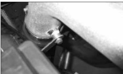
25. Align the weld-on stud on the tube with the mounting bracket and secure using an M6 bolt, flat metal washer and wave washer supplied as shown. Don't fully tighten yet!
