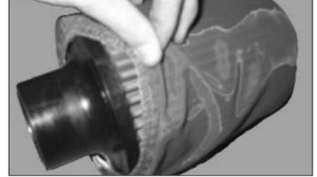
33. Fit the K&N Drycharger over the K&N Filter as shown. **NOTE:** The Drycharger's water repellent properties will last up to 2 years. See parts list to re-order Drycharger if necessary.
