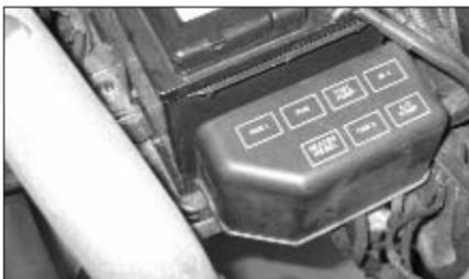
43. Re-install the relay box cover as shown.
