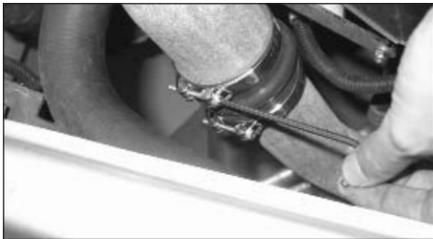
36. Line up the intake tube and cold air extension tube in the silicone hump hose and fully tighten the hose clamps as shown.
