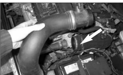
6. Undo the indicated hose clamp and remove the intake tube and MAS as shown.
