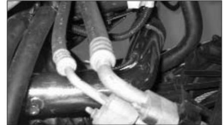
30. From underneath the vehicle, feed the cold air extension tube (the end without the weld-on stud) into the silicone hump hose as shown but don't tighten the hose clamp yet.
