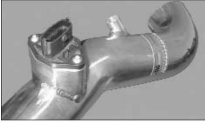
22. Install the MAS into the intake tube using the M5 bolts supplied as shown. **NOTE:** Before installing the MAS, clean the inside of the tube using water and a towel.
