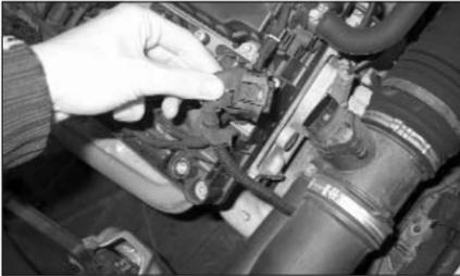
3. Unclip the electrical connector from the Mass Air Sensor (MAS) as shown.
