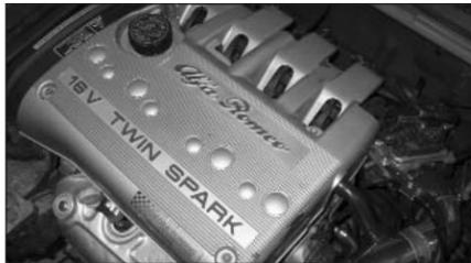
41. Remove the oil filler cap, re-install the engine cover using its original hardware as shown and place back the oil filler cap.
