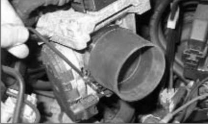
19. Fit the stepped silicone sleeve to the throttle body using the #44 hose clamp supplied as shown.
