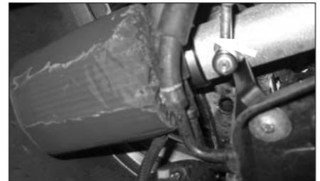
35. Adjust the filter/cold air extension tube to clear all surrounding parts; now fully tighten all hardware securing the cold air tube and its mounting bracket as shown.
