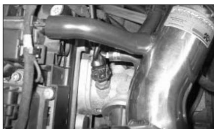
40. Install the breather hose supplied between the vent on the engine and the vent on the intake tube as shown; trim as necessary to eliminate sharp bends in the hose.
