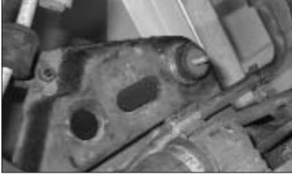
26. Remove the rubber grommets from the air box mounting holes. Place a large washer and a rubber stud supplied over the indicated air box mounting hole as shown.
