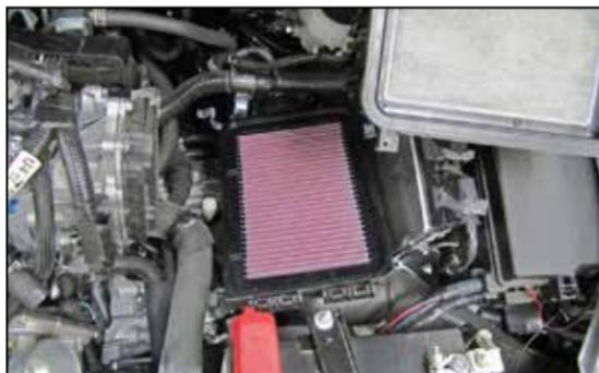
4. Release the clips that secure the upper air filter housing, lift up the housing and remove the factory air filter. Install the provided K&N® air filter and then reinstall the upper housing and secure with the factory retaining clips.
