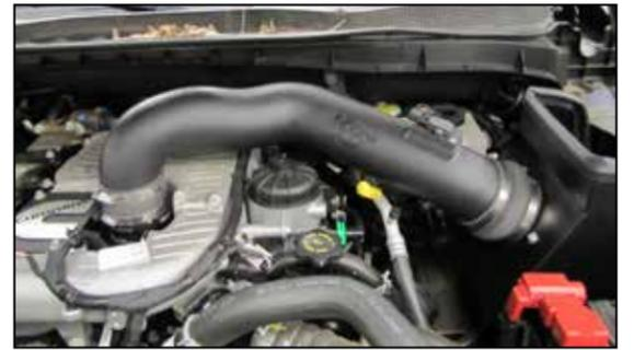
17. Install the K&N® intake tube into the coupler at the filter adapter and then into the hose at the turbo inlet, adjust the tube for best fit and then secure with the provided hose clamps.
