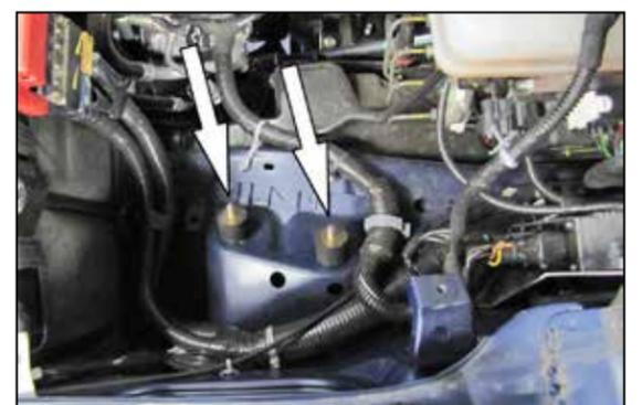
5. Install the two provided rubber mounted studs into the air filter housing mounting locations as shown.
