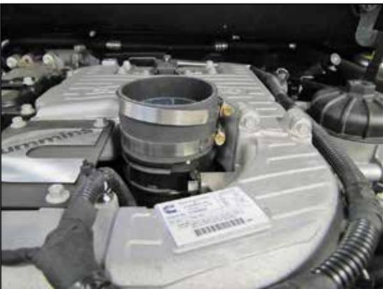
11. Install the provided coupler hose (08698) onto the turbo inlet and secure with the provided hose clamp.
