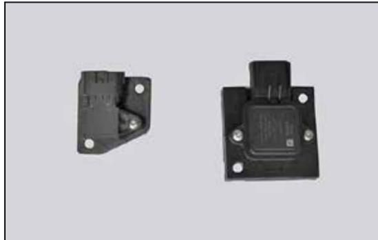
15. Install the sensors into the K&N® adapters using the provided hardware.
