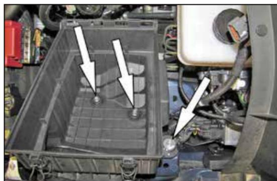
4. Loosen the three bolts that secure the lower air filter housing and then remove the housing from the vehicle.
