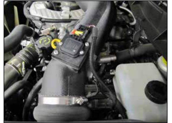
18. Reconnect the mass air sensor and inlet air temperature sensor electrical connections.
