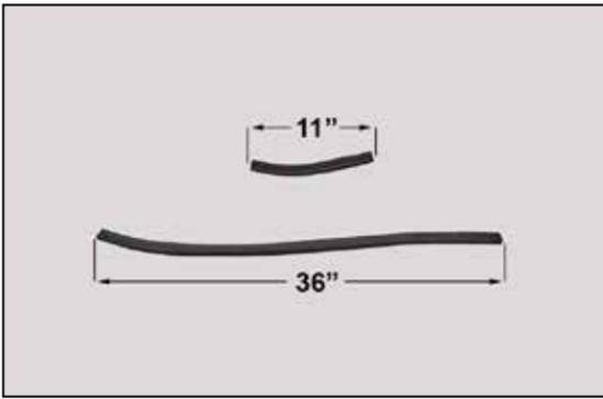
7. Cut the provided edge trim into two sections, one section will be 11" long and the other section will be 36" long.
