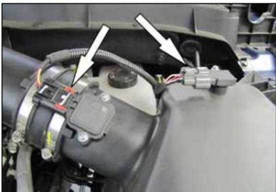
2. Disconnect the mass air sensor and inlet air temperature sensor electrical connections.
