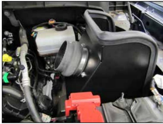
12. Install the provided coupler hose (08418) onto the filter adapter and secure with the provided hose clamp.
