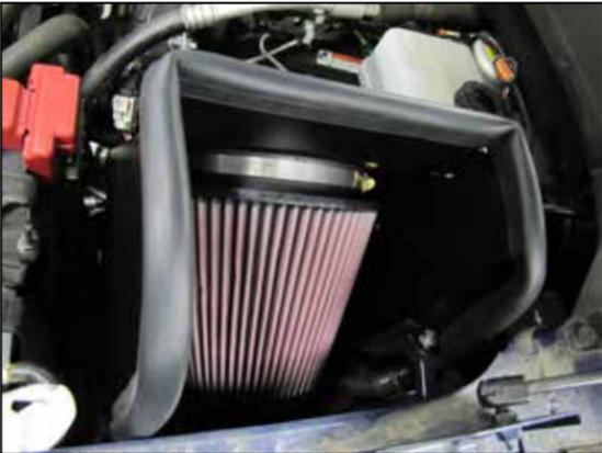
10. Install the air filter onto the filter adapter and secure with the provided hose clamp. Secure the heat shield to the remaining mount with the hardware provided.
