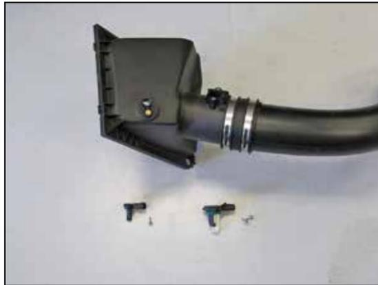
14. Remove the two sensors from the stock air filter housing.
