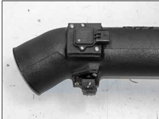
16. Install the sensor assemblies into the K&N® intake tube and secure with the provided hardware.
