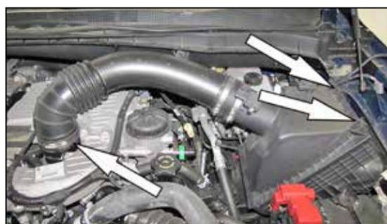
3. Loosen the hose clamp that secures the intake tube to the turbo inlet and then release the two clam shell clips that secure the upper air filter housing. Remove the upper air filter housing and intake tube from the vehicle.
