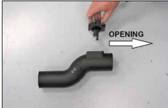
15. Install the mass air sensor assembly into the K&N intake tube and secure with the provided hardware.
