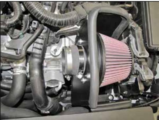
11. Install the coupling hose (084036) onto the filter adapter and secure with the provided hose clamp.
