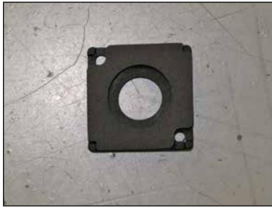
12. Install the provided gasket onto the mass air sensor adapter.
