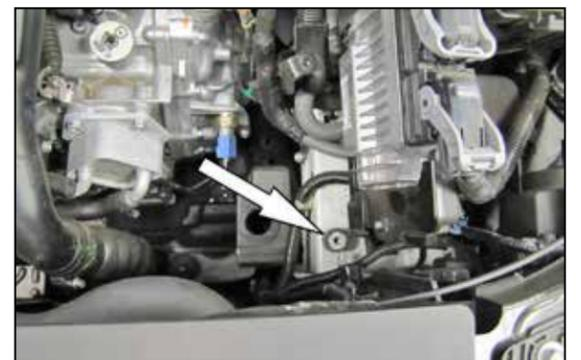
5. Install the provided rubber mounted stud onto the inner fender air filter housing mounting location.
