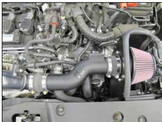
16. Install the K&N® intake tube assembly into the coupling hoses, adjust the tube for best fit and then secure with the provided hose clamps.
