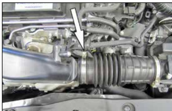
4. Loosen the hose clamp that secures the intake hose to the turbo inlet pipe and then remove the air filter housing and hose assembly.
