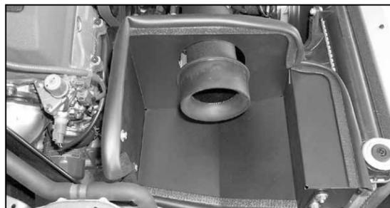
32. Install the radiused adapter onto the K&N® intake tube.
