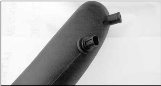
26c. Remove the air temperature sensor from the stock intake tube and install it into the grommet installed in the K&N® intake tube in the previous step as shown.
