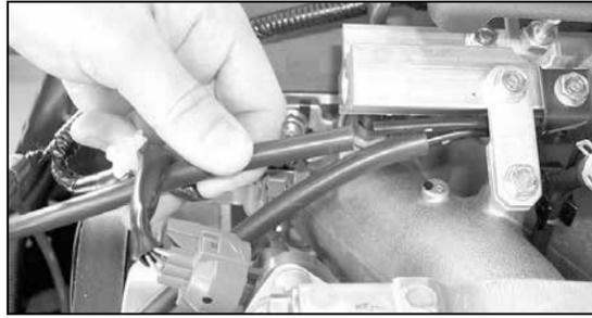
17. On vehicles equipped with air injection pump, attach the check valve vacuum line to the check valve hard line (upper hard line).
