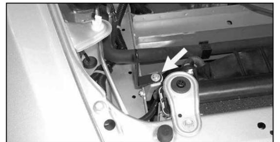
23. Using the provided hardware, install the small "L" bracket onto the vehicle as shown.
