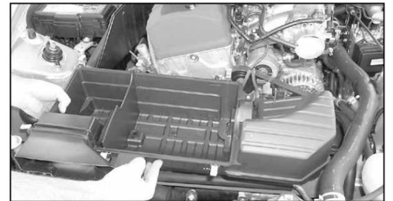
7. Loosen and remove the 3 bolts that secure the air cleaner base, then remove the air cleaner base.
