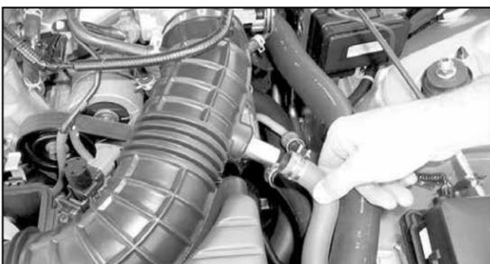
3. On vehicles equipped with air injection pump, detach the air injection pump hose from the stock intake tube.
