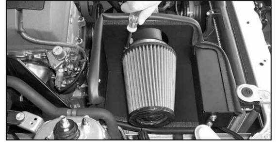
33. Install the K&N® air filter onto the K&N® intake tube and secure with the provided hose clamp.
