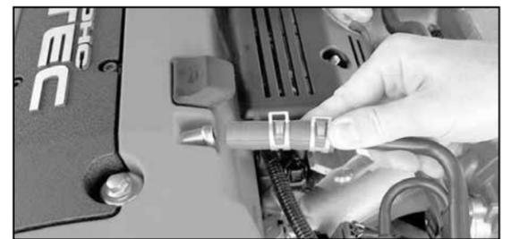
8. Remove the crank case vent hose from the vent on the cam cover.
