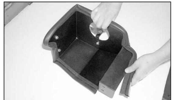
22. Install the edge trim to the heat shield assembly.
