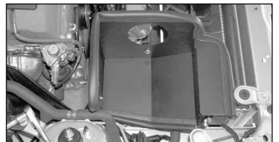
24. Using the provided hardware, install the heat shield assembly and secure the brackets to the original air box mounting locations.
