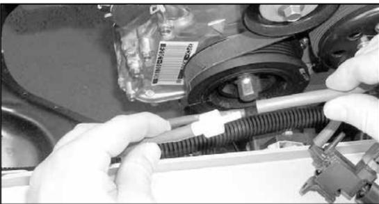
12. On vehicles equipped with air injection pump, detach the vacuum hose from the air control vacuum check valve.
