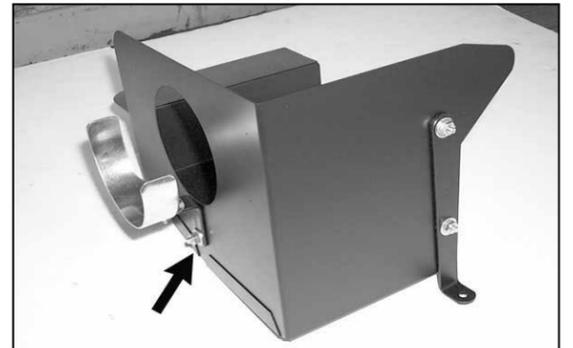
21. Using the provided hardware attach the saddle bracket assembly to the heat shield.
