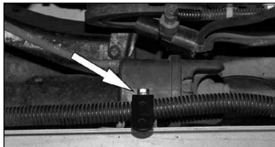
17b. Using the provided hardware, install the provided bracket (083155) along with the provided spacer and the factory vacuum canister.
