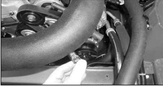
26a. On vehicles equipped with an air temperature sensor, position the air temperature sensor wiring harness on the intake tube for best fit and mark the position on the intake tube with a marker for drilling.
