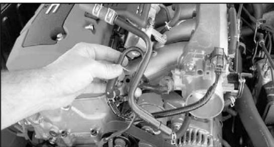
13. Remove the pipe assembly.
