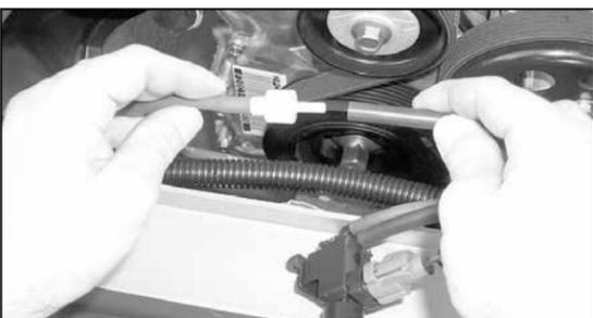
15. On vehicles equipped with air injection pump, attach the provided 4mm (short) vacuum hose to the check valve.
