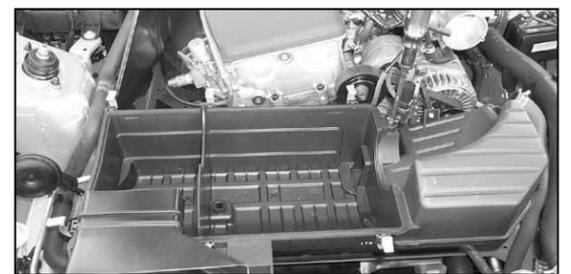
6. On vehicles equipped with air control solenoid, loosen and remove the screw and push clip that secures the air control solenoid valve to the air box base.
