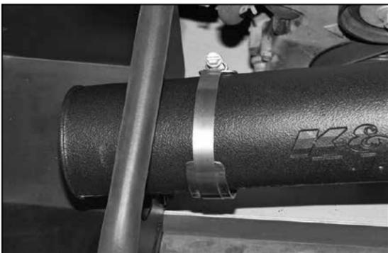
27. Install the K&N® intake tube onto the throttle body and align it with the saddle clamp on the heat shield and secure with the provided hose clamps.
