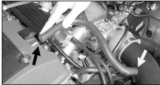
29. Attach the provided 1/2" hose to the crank case vent on the cam cover, then attach the other end to the vent on the K&N® intake tube.
