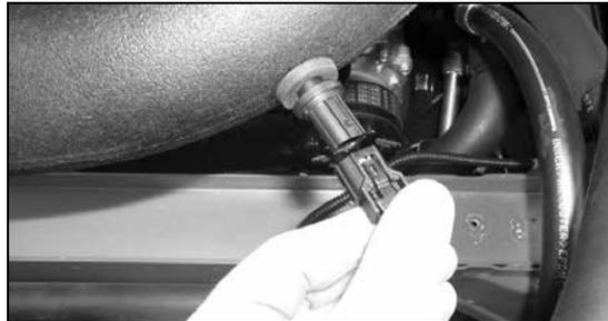
28b. On vehicles equipped with an air temperature sensor, reconnect the air temperature sensor electrical connection as shown.
