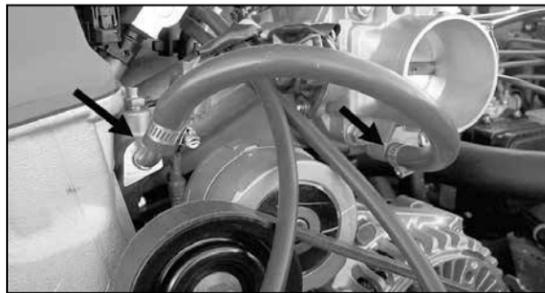
18. Attach the provided 1/4" reinforced hose to the fitting on the intake manifold and the fitting on the underside of the throttle body.
