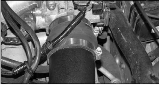
26. Install the intake K&N® tube and secure the hump hose to the throttle body as shown.
