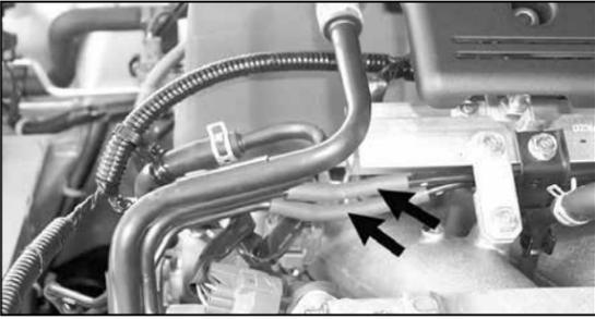
10. Detach the air control valve vacuum hose and the air control solenoid vacuum hose from the hard lines.
