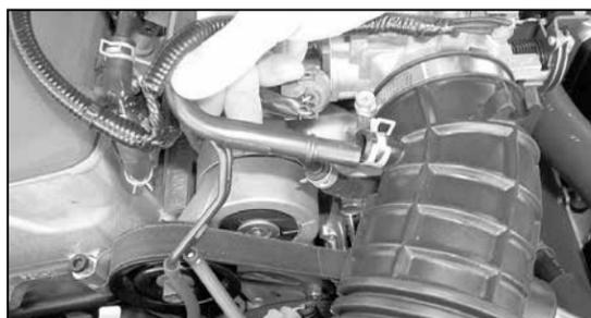
4. Remove the crank case vent hardline from the stock intake tube.
