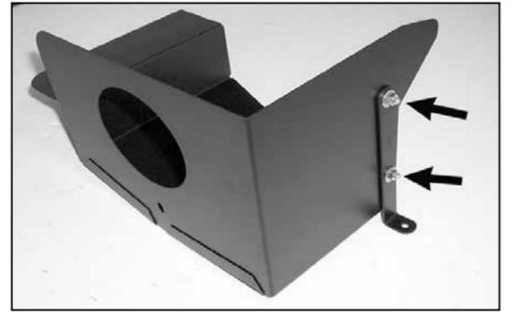
20. Using the provided hardware attach the long "L" bracket to the heat shield.
