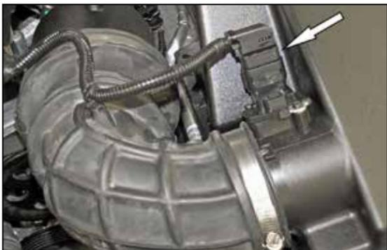
2. Disconnect the mass air sensor electrical connection and unhook the wiring harness from the intake tube.
