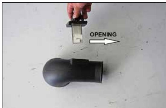
16. Install the mass air sensor assembly into the K&N® intake tube and secure with the provided hardware.
