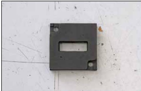
13. Install the provided gasket onto the bottom of the mass air sensor adapter.
