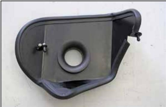
8. Install the edge trim onto the heat shield as shown. Some trimming of the edge trim will be necessary.
