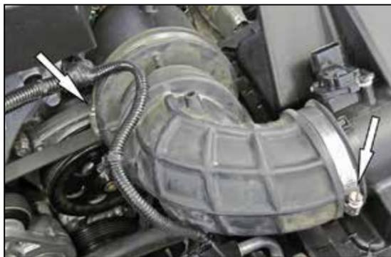
3. Loosen the two hose clamps that secure the intake tube to the turbo inlet and air filter housing. And then remove the intake tube from the vehicle.
