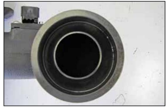
17. Install the air diffuser into the K&N® intake tube so the radiused surface is located inside the tube.
