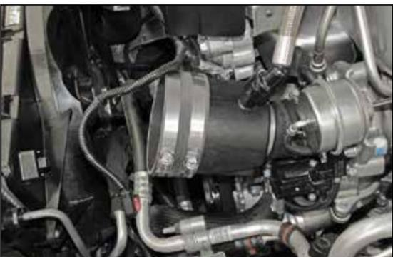
11. Install the provided coupler hose (08540) onto the turbo inlet chamber and secure with the provided hose clamp.
