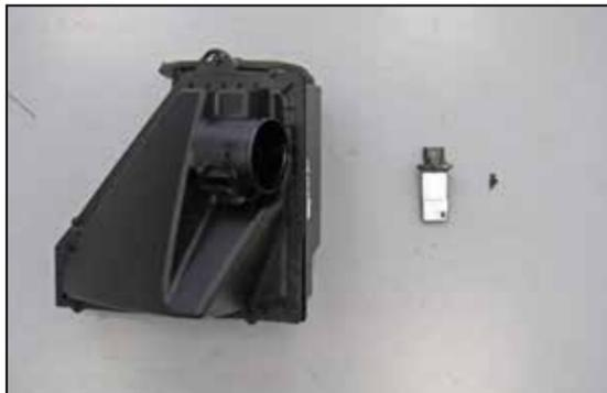
14. Remove the mass air sensor from the factory air filter housing.
