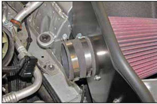
12. Install the provided coupler hose (08711) onto the filter adapter and secure with the provided hose clamp.
