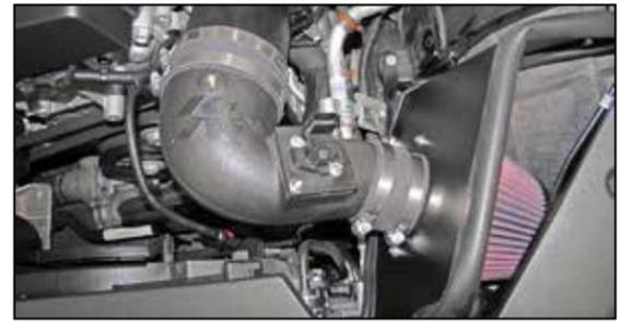
18. Install the K&N® intake tube into the hose at the filter adapter and then into the hose at the turbo chamber, adjust the tube for best fit and then secure with the provided hose clamps.
