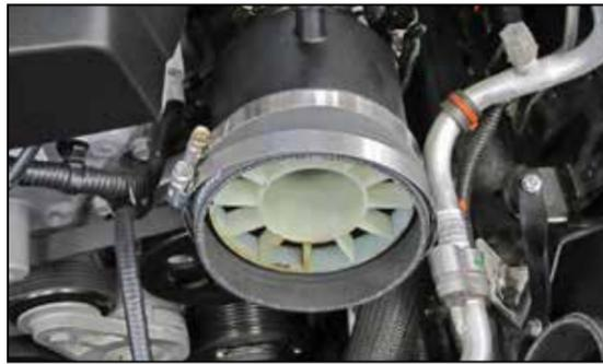
12. Install the provided coupler hose (08540) onto the turbo inlet chamber and secure with the provided hose clamp.
