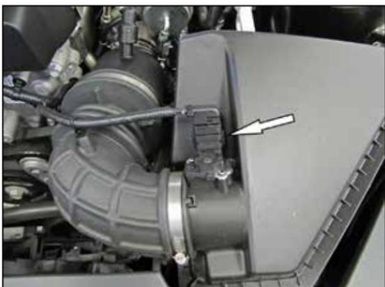
2. Release the locking tab and then disconnect the mass air sensor electrical connection and unhook the wiring harness from the intake tube.
