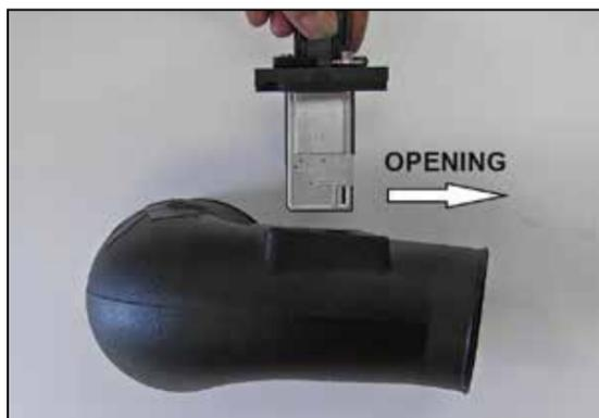
16. Install the mass air sensor assembly into the K&N® intake tube as shown with the opening of the sensor towards the inlet of the intake tube. Secure the assembly with the provided hardware.
