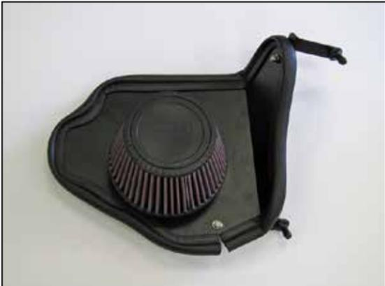
9. Install the K&N® air filter onto the filter adapter and secure with the provided hardware.
