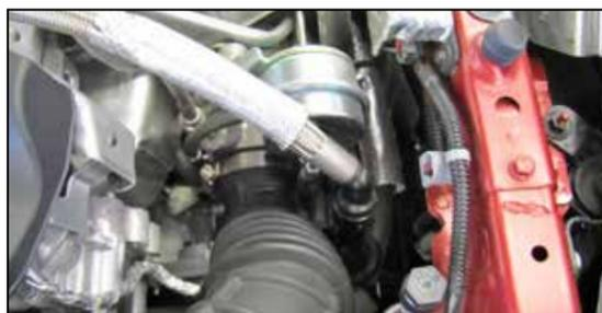
3. Disconnect the crank case vent hose.
