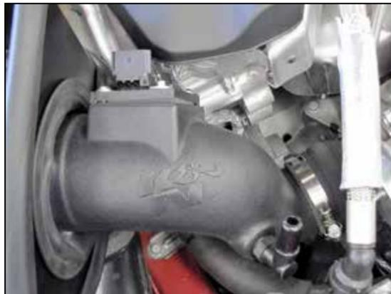
16. Install the K&N® intake tube assembly through the opening in the heat shield and then onto the Turbo inlet. Adjust the tube and heat shield for best fit and then secure them with the hose clamp and hardware.
