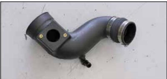
11. Install the 90° NPT vent fitting into the K&N® intake tube as shown.
