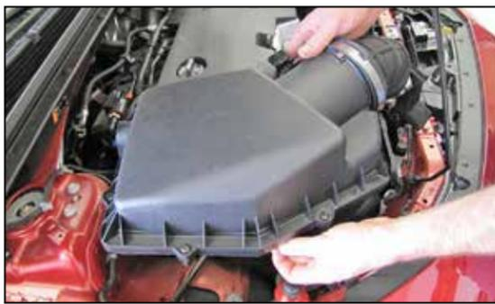
4. Loosen the hose clamp securing the intake tube to the turbo inlet. Lift up the air filter housing, detach the intake hose from the turbo and then remove the complete intake system from the vehicle.
