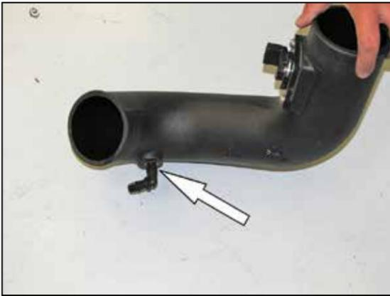
22. Install the provided 90° vent fitting into the K&N® intake tube as shown.
