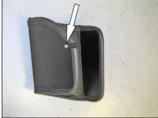
12. Install the provided heat shield mounting bracket (07805) onto the heat shield as shown using the provided hardware.
