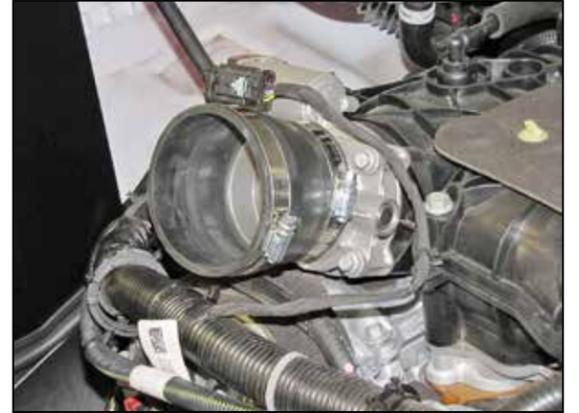
17. Install the provided step coupler (08724) onto the throttle body and secure with the provided hose clamp.
