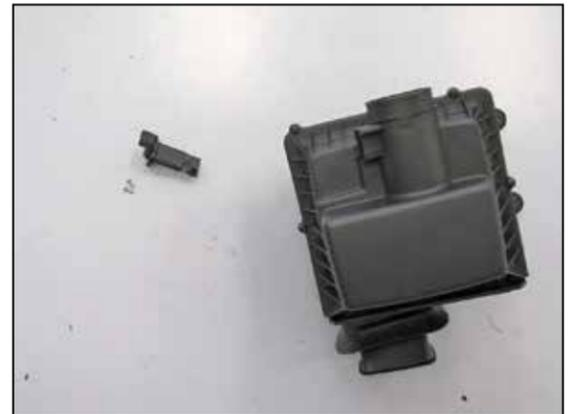
19. Remove the mass air sensor from the factory air filter housing.
