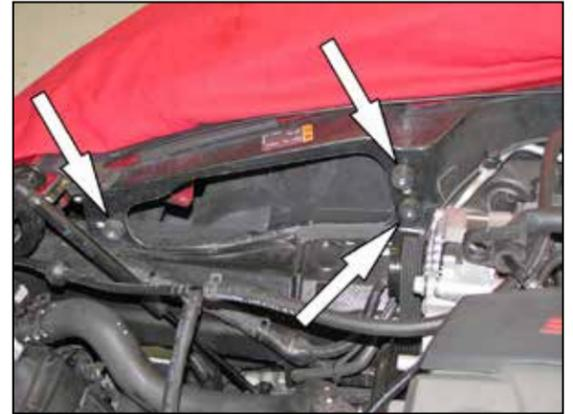
14. Install the three provided rubber mounted studs onto the heat shield mounting location as shown.
