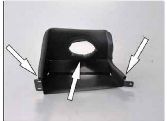
16. Install the 16" section into the hole of the heat shield and install the 27" section around the perimeter of the heat shield as shown.
