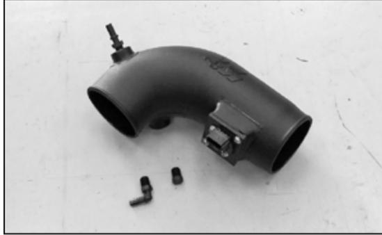
24. Install the provided vent fittings into the into the K&N intake tube as shown.
