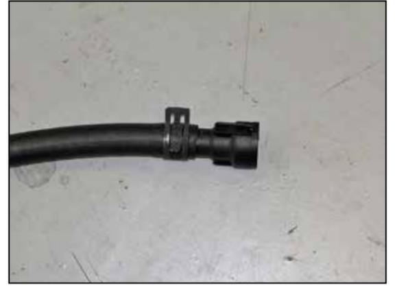
27. On vehicles that are equipped with a "Dry Sump" oiling system, assemble the provided crank case vent hose (08635) and quick disconnect fitting and clamp as shown.
