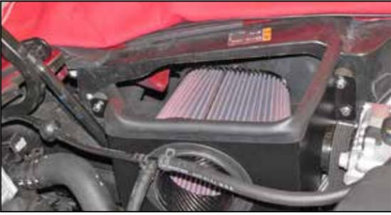
18. Install the heat shield assembly onto the rubber mounted studs and secure with the provided hardware.
