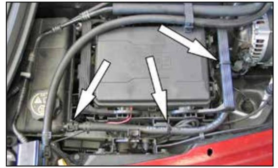
13. Install the provided coolant hose assembled from step #10 onto the expansion tank. Route the coolant hose and then attach the open end onto the TEE fitting and secure with the provided spring clamp. Use the provided tie wraps to secure the coolant hose.
