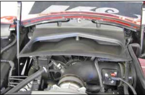
33. Reinstall the air extraction duct and secure with the factory hardware.
