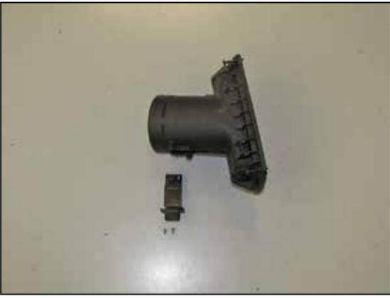
20. Remove the two screws securing the mass air sensor to the factory housing and then remove the sensor from the housing.
