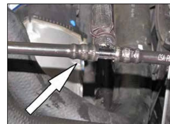
12. Using a razor knife, cut the plastic hose at the TEE fitting where shown. Separate the plastic hose from the TEE fitting.
