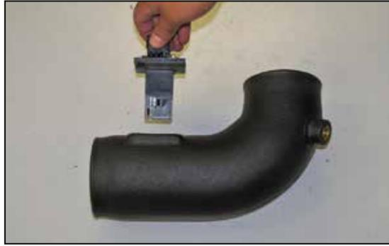
23. Install the mass air sensor assembly into the K&N intake tube and secure with provided hardware.
