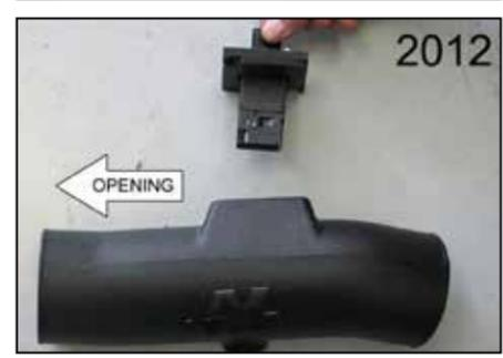
19. Install the mass air sensor assembly into the K&N® intake tube as shown and secure with the provided hardware.
