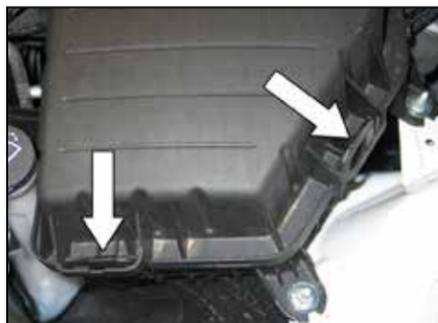
6. Unlatch the upper air box clips and remove the upper air box and intake tube assembly.
