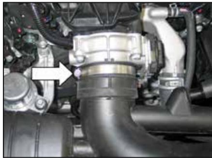
5. Loosen the hose clamp that secures the intake hose to the throttle body.
