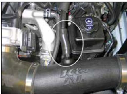
22. Remove the 90° vent hose from the crank case vent tube. Install the provided silicone vent hose and install it onto the fitting installed into the K&N® intake tube. Trim the vent hose for proper fit.
