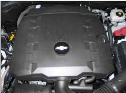
2. Remove the oil fill cap, lift up and remove the engine cover. Reinstall the oil cap.
