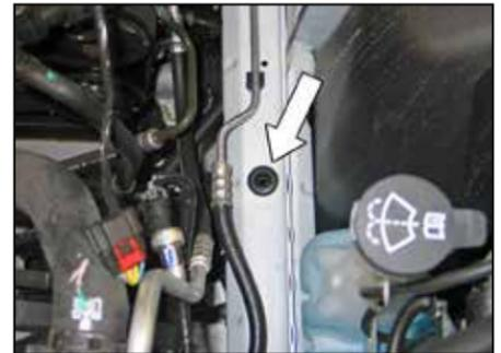
8. Remove the air box mounting grommet shown on the frame rail.
