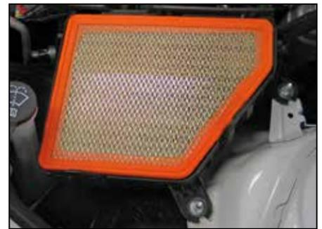
7. Remove the lower air box mounting nuts, then remove the lower air box assembly. **NOTE: K&N Engineering, Inc., recommends that customers do not discard factory air intake.**
