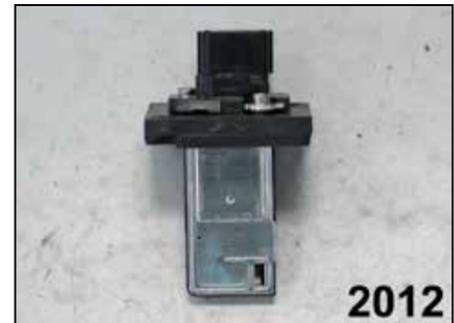
18. Install the mass air sensor into the mass air sensor adapter and secure with the provided hardware.
