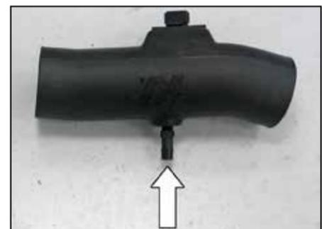
20. Install the provided vent fitting into the K&N® intake tube as shown.
