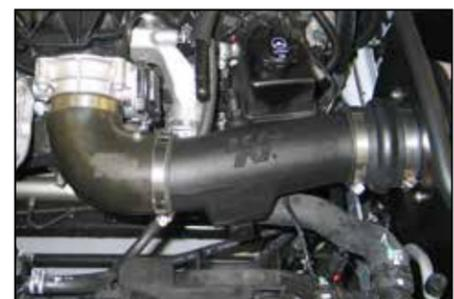
21. Install the provided silicone hose (08629) onto the K&N® intake tube as shown. Install the K&N® intake tube assembly onto the throttle body and hump hose attached to the filter adapter. Adjust the intake tube in the hoses for proper fit, once proper fit is achieved secure the tube with the provided hose clamps.
