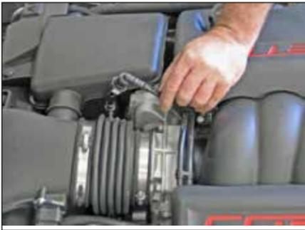
2. Unlock and disconnect the crankcase vent tube from the intake tube as shown.
