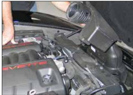
5. Lift up and remove the complete stock intake system from the vehicle as shown.
