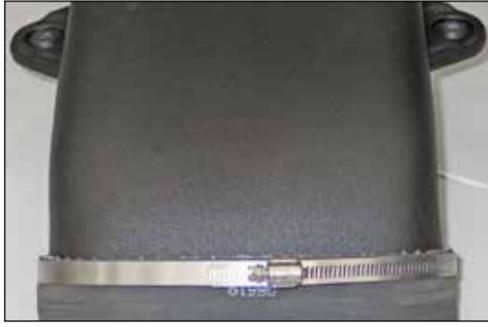
15. Install the provided silicone hose (08619) onto the K&N® intake tube and secure with the provided hose clamp.
