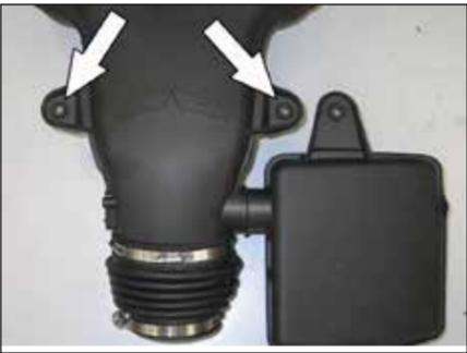
13. Remove the two intake tube mounting grommets from the stock intake tube.
