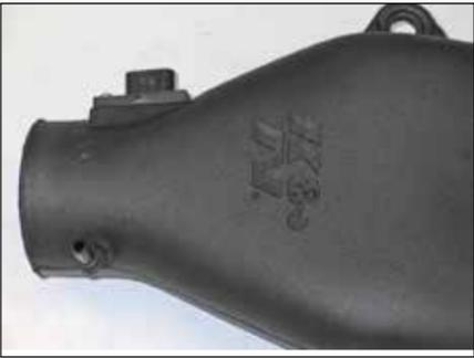
12. Install the factory crankcase vent fitting into the grommet as shown.
