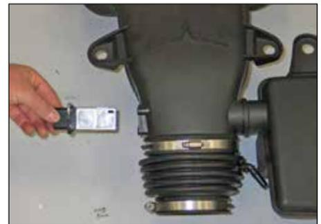
7. Remove the two screws which secure the mass air sensor to the stock intake tube and then remove the mass air sensor from the intake tube as shown.
