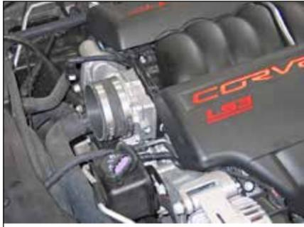
17. Install the provided silicone hose (08761) onto the throttle body and secure with the provided hose clamp.
