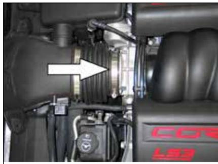
4. Loosen the hose clamp which secures the stock intake tube to the throttle body.
