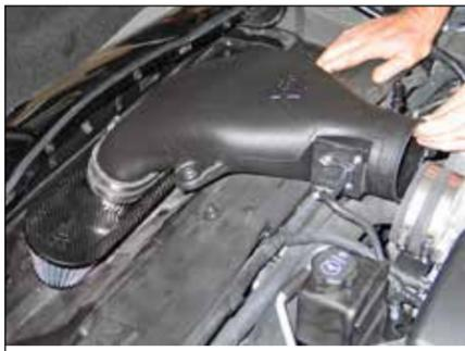
18. Install the K&N® intake assembly on top off the radiator assembly and then connect the mass air sensor electrical connection as shown.
