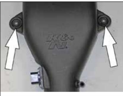
14. Install the two mounting grommets into the K&N® intake tube.
