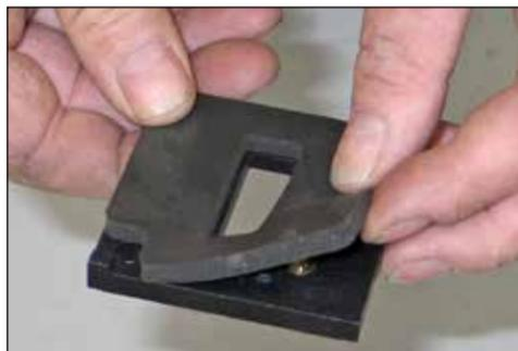
6. Install the provided gasket onto the mass air sensor adapter as shown.
