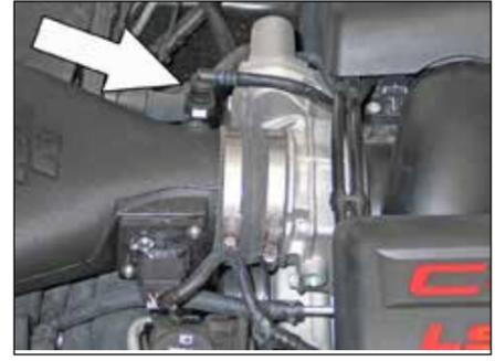
19. Install the K&N® intake assembly into the silicone hose on throttle body and onto the mounting studs. Secure with the provided hose clamp. Reconnect the crank case vent line.
