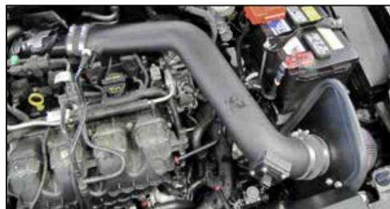
18. Install the K&N® intake tube assembly into the coupler at the turbo inlet and then into the coupler at the filter adapter, adjust the tube for best fit and then secure with the provided hose clamp.
