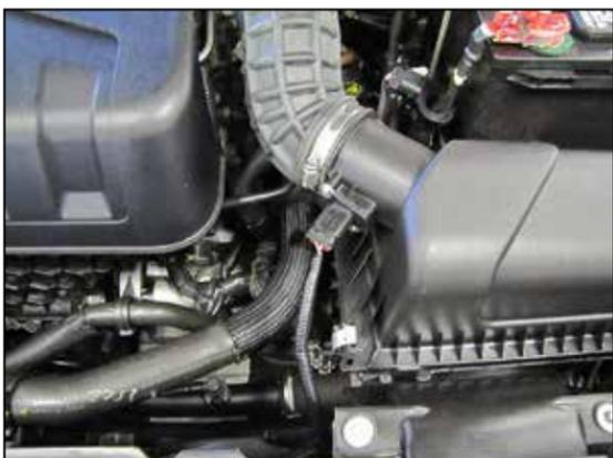
2. Release the red locking tab and then disconnect inlet air temperature sensor electrical connection.
