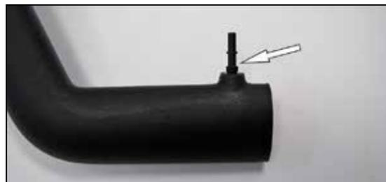
17. Install the provided quick disconnect fitting into the K&N® intake tube as shown.
