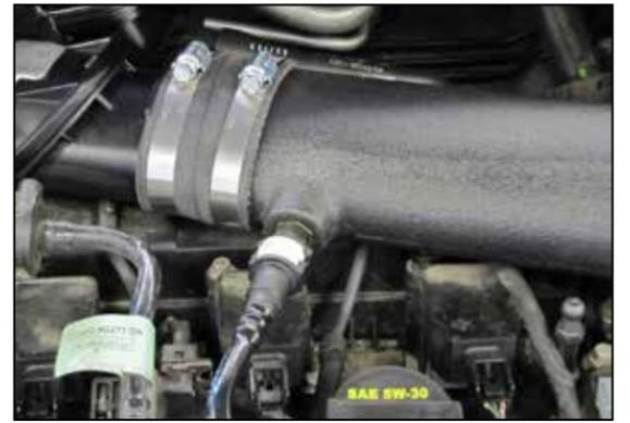
20. Connect the EVAP vent line to the quick disconnect fitting installed into the K&N® intake tube.
