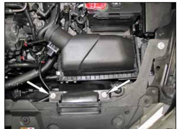
6. Remove the two bolts that secure the fresh air duct to the core support then lift up and remove the complete air filter housing from the vehicle.
