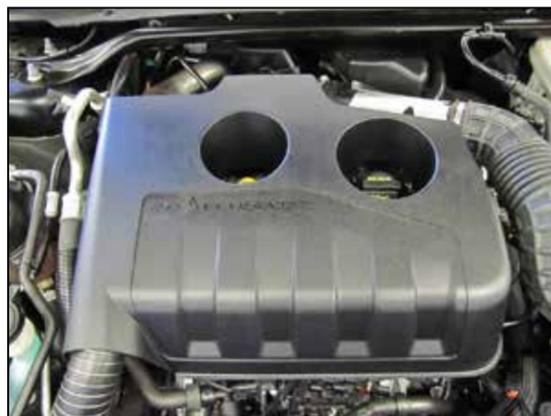
3. Lift the engine cover and remove it from the vehicle.
