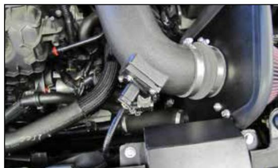
19. Reconnect the Inlet air temperature electrical connection.
