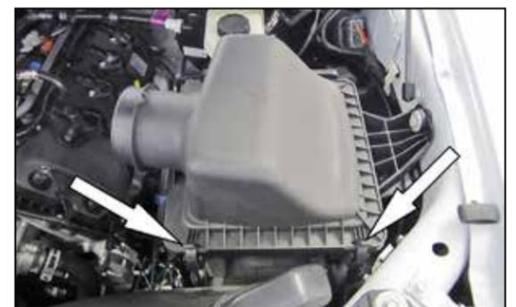
5. Release the two clips securing the upper air filter housing and then remove the upper filter housing and stock air filter.
