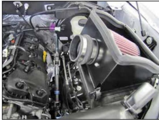
12. Install the provided coupling hump hose (08639) onto the filter adapter and secure with the provided hose clamp.
