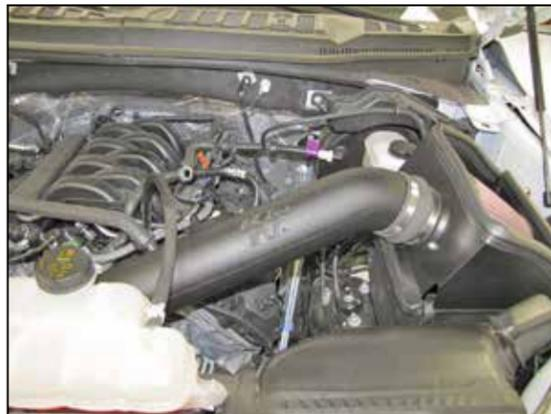
15. Install the K&N® intake tube into the coupling hose at the filter adapter and then into the hose at the throttle body, adjust the tube for best fit and then secure with the provided hose clamps.
