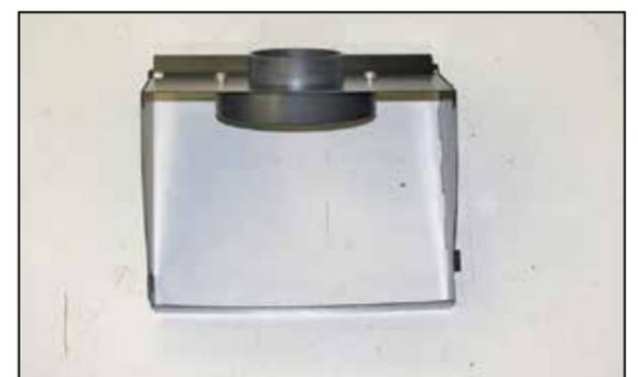
6. Install the filter adapter into the K&N® heat shield and secure with provided hardware.
