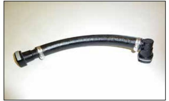
16A. On some later models it may be necessary to assemble the crank case vent hose assembly with the provided parts and install due to the manufacturer changing the position on the valve cover port. Install the assembly with the 90° fitting attached to the valve cover port.
