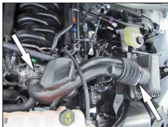
3. Loosen the hose clamps at the throttle body and filter inlet that secure the factory intake tube.
