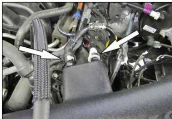
16. Connect the factory EVAP and Crank case vent lines to the fittings on the K&N® intake tube.
