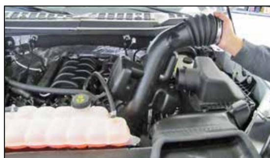
4. Unhook the coolant line from the intake tube and then remove the intake tube from the vehicle.
