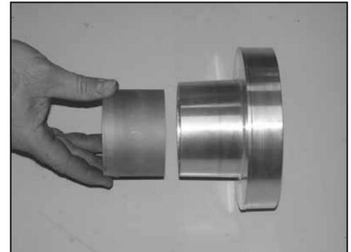
22. Vehicles that come equipped with Hydrocarbon trap, place the Hydrocarbon trap into the filter adapter as shown.
