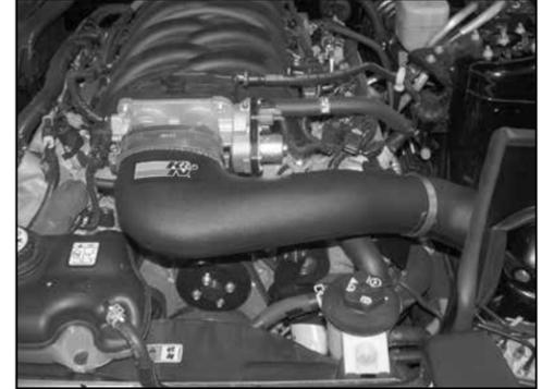
19. Install the K&N® intake tube into the silicone hose at the throttle body and onto the saddle bracket assembly then secure with the provided hose clamps as shown.
