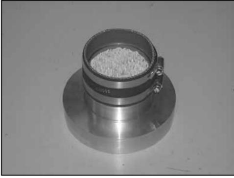
23. Install the silicone hose (08630) onto the filter adapter and secure with the provided hose clamp as shown.
