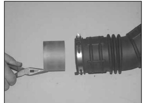
21. Vehicles that come equipped with Hydrocarbon trap, use a pair of needle nose pliers, to remove the Hydrocarbon trap from the stock intake tube as shown.
