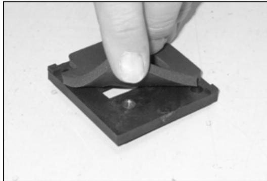
17. Install the provided gasket to the back of the K&N® mass air sensor adaptor plate as shown.
