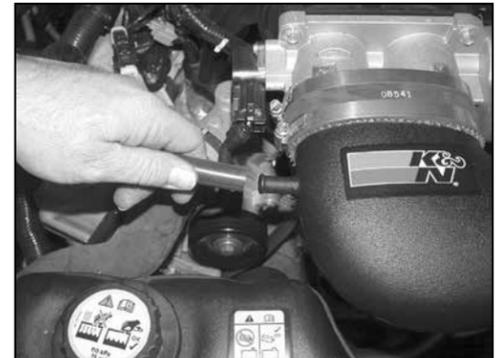
20. Install the supplied vent hose onto the vent port on the valve cover and secure with the provided hose clamp, then onto the K&N® intake tube as shown.
