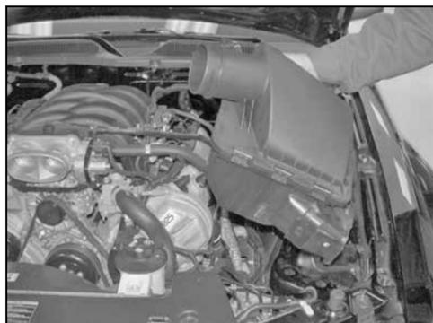
6. Remove the air box assembly as shown. **NOTE: K&N Engineering, Inc., recommends that customers do not discard factory air intake.**
