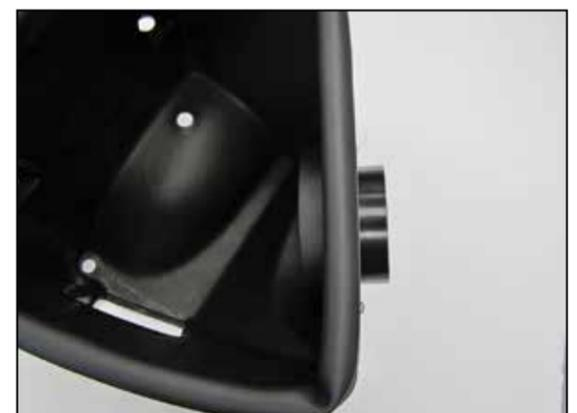
6. Install the filter adapter into the K&N® air filter housing and secure with the provided hardware.
