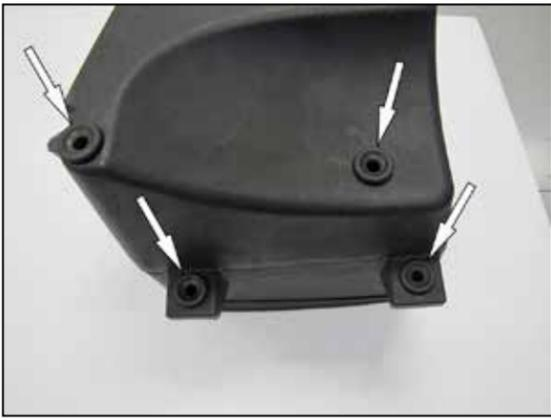
7. Remove the four mounting grommets from the factory air filter housing and install them into the K&N® housing as shown.
