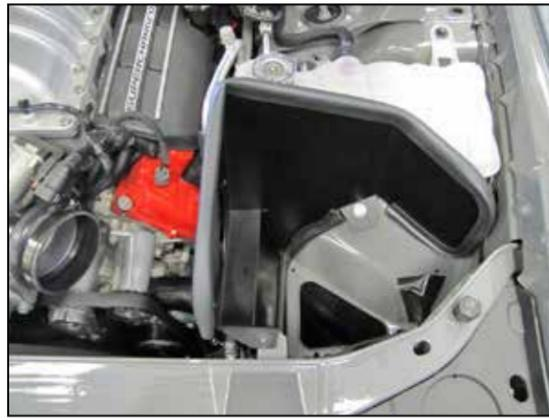
12. Install the provided coupling hose (KITHUMPHS12) onto the throttle body and secure with the provided hose clamp. Set the heat shield into position on the inner fender but do not secure at this time.
