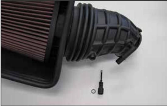
9. Remove the inlet air temperature sensor from the factory intake tube.
