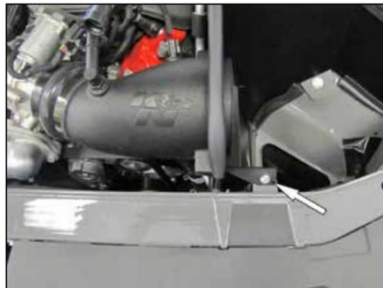
14. Secure the heat shield to the core support with the provided hardware then secure the intake tube with the provided hose clamp.
