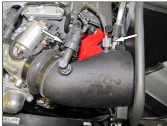
15. Reconnect the inlet air temperature sensor electrical connection and crank case vent line.
