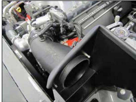
13. Install the K&N® intake tube into the coupling hose and heat shield and secure with the provided hardware to the heat shield.
