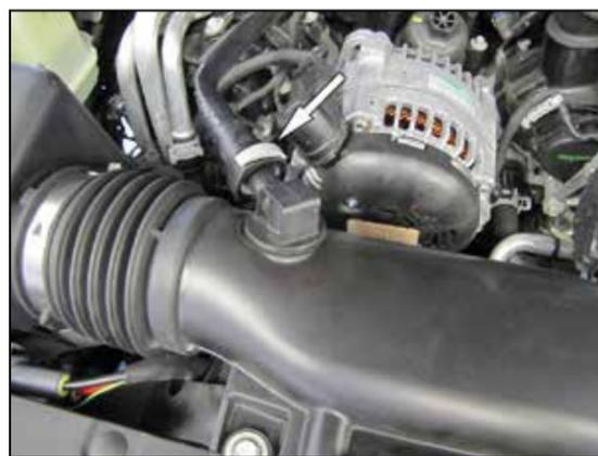
3. Disconnect the crank case vent line.
