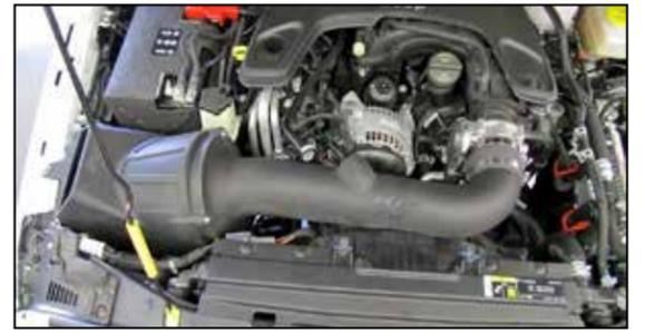
17. Install the K&N® intake assembly into the hose at throttle body first, then engage the K&N® airbox mounts into the factory airbox mounting location. Secure K&N® intake assembly with provided clamp.
