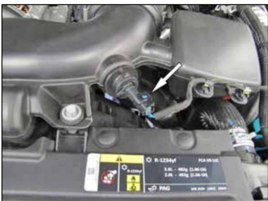
2. Disconnect the inlet air temp electrical connector.
