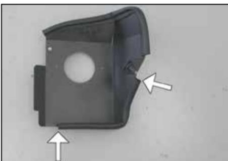
11. Install the provided shorter edge trim onto the bottom of the heat shield as shown.
