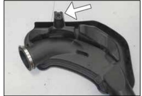
19. Remove the intake plenum mounting grommet from the intake plenum.
