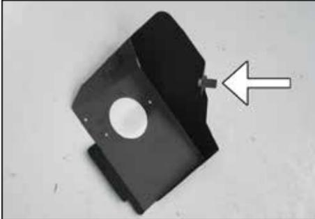
8. Install the inserted nut onto the heat shield using the provided hardware as shown.
