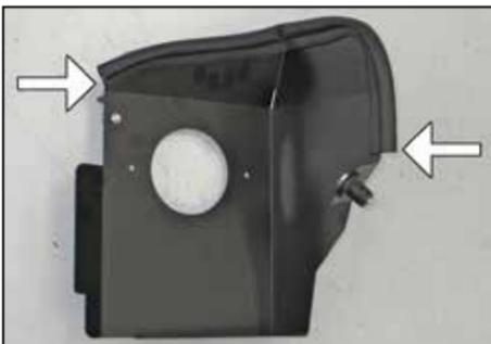
10. Install the provided longer edge trim onto the top of the heat shield as shown.
