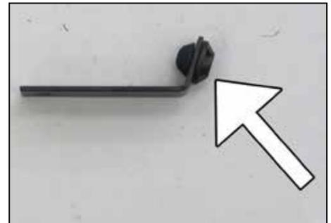
20. Install the mounting grommet from the intake plenum into the provided tube bracket as shown.
