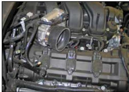
15. Install the provided silicone hose (084091) onto the throttle body and secure with the provided hose clamp.
