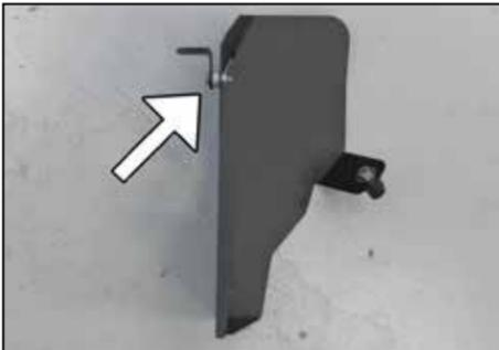
9. Install the heat shield mounting bracket (070066A) onto the heat shield as shown using the provided hardware and spacer.
