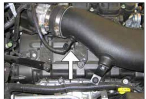
22. Reconnect the inlet air temperature sensor electrical connection.
