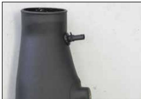
17. Install the provided grommet and inlet air temperature sensor into the K&N® intake tube as shown.
