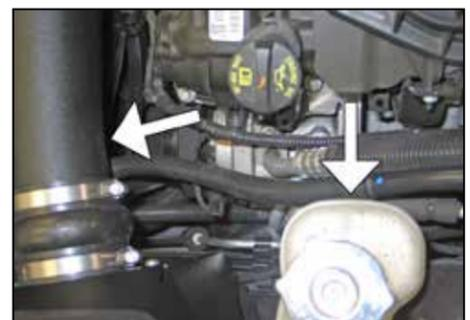
23. Install the provided silicone hose onto the factory crank case vent tube and then connect the open end to the 90° fitting installed into the K&N® intake tube.
