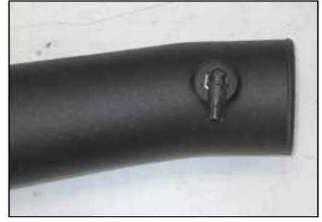
18. Install the 90° NPT fitting into the K&N® intake tube as shown.
