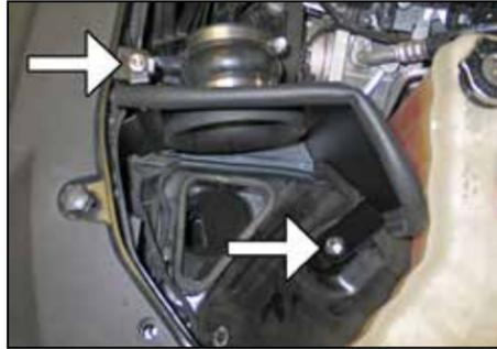
14. Install the heat shield assembly onto the inner fender; secure the mounting bracket to the factory air box mounting location and secure with the provided hardware. Place the insert nut into the hole in the inner fender and tighten the bolt to secure.
