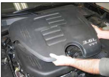
2. Lift up and remove the engine cover.
