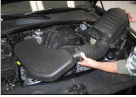
7. Remove the complete stock intake system from the vehicle.
