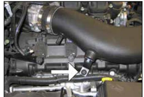
21. Install the K&N® intake tube into the silicone hump hose and then into the throttle body silicone hose. Install the tube bracket onto the mounting stud and secure it to the K&N® intake tube with the provided hardware. Tighten the hose clamps at this time.
