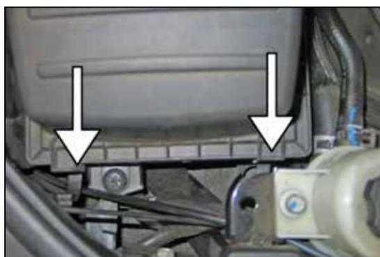
6. Release the two upper airbox retaining clips.
