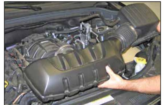
7. Remove the upper airbox and intake tube assembly.
