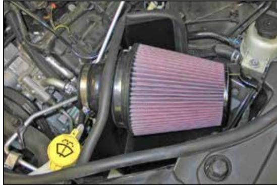
16. Install the K&N® filter onto the adapter and secure with the provided hose clamp.
