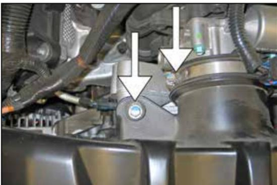
3. Remove the intake plenum mounting bolt shown and loosen the intake tube hose clamp.
