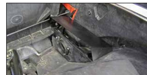
13. Install the fresh air scoop onto the tube mount using the provided hardware, then reinstall the assembly to the body using the factory bolts from the previous step.
