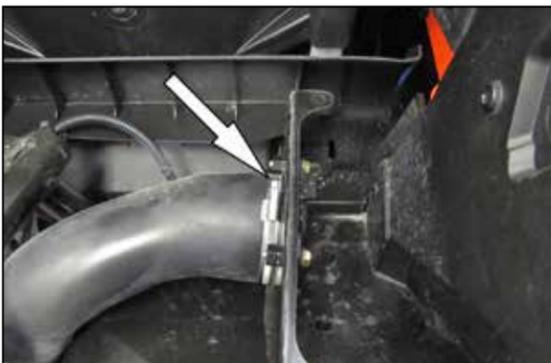
9. Loosen the hose clamp that secures the fresh air intake hose to the mount and then disconnect the fresh air hose.
