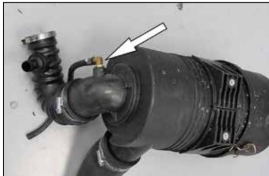
15. Remove the waste gate hose and fitting from the factory intake tube.
