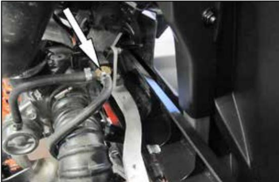
7. Cut the pinch clamp securing the waste gate valve vacuum hose and then disconnect the vacuum hose from the vacuum switch.
