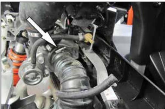
8. Loosen the hose clamp that secures the intake hose to the turbo inlet and then disconnect the hose from the turbo.
