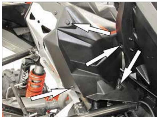
30. Reinstall the charge air cooler cover and secure with the factory bolts.
