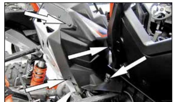
5. Remove the four bolts that secure the right side charger air cooler cover and then remove the cover.
