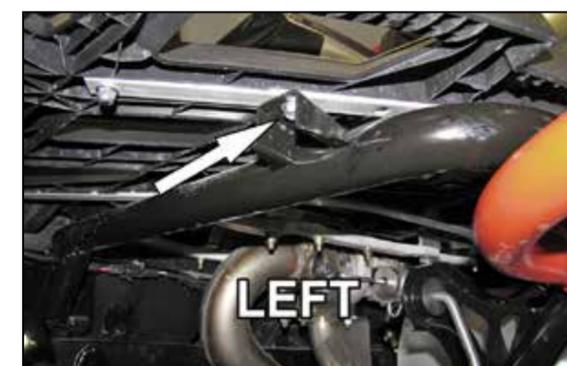
3. Remove the bolts that secure the package tray from the underside.
