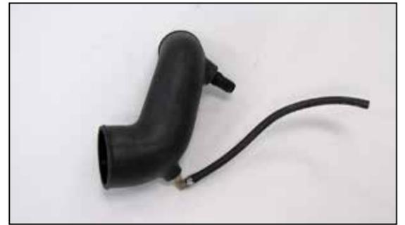
16. Install the waste gate hose and fitting along with the provided crank case vent hose fitting into the K&N® intake tube as shown.
