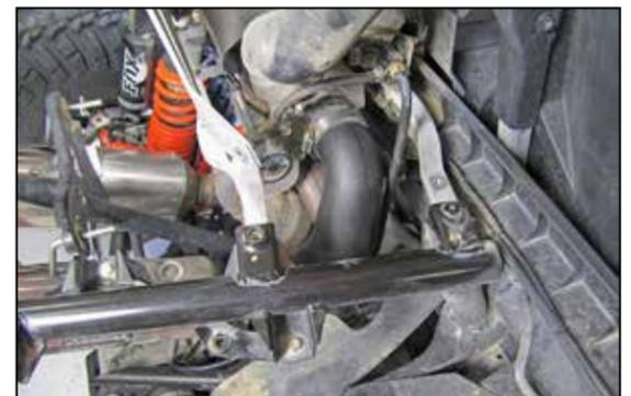
19. Install the K&N® intake tube into the coupler hose and secure with the provided hose clamp. Connect the waste gate vacuum hose to the vacuum switch and secure with the provided tie wrap.
