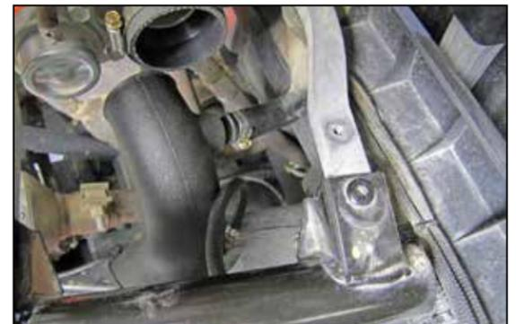
18. Connect the crank case vent hose to the fitting installed into the K&N® intake tube and secure with the provided hose clamp.
