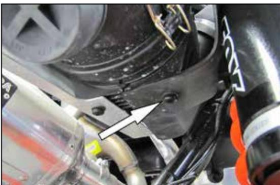
10. Remove the three bolts that secure the air filter assembly.
