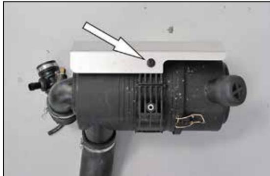
14. Remove the bolt that secures the heat shield to the air filter assembly and remove the heat shield.
