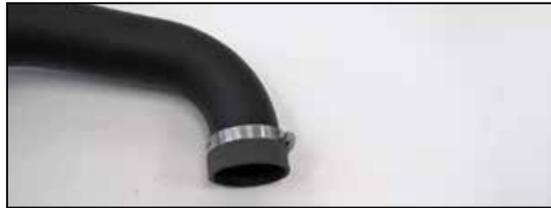
28. Install the provided coupler hose (08179) onto the K&N® intake tube and secure with the provided hose clamp.
