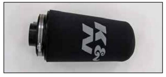
20a. Install the provided foam wrap onto the K&N® air filter.
