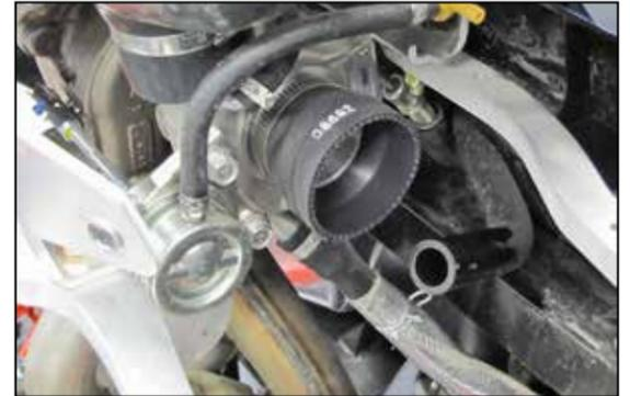
17. Install the provided coupler hose (08682) onto the turbo inlet and secure with the provided hose clamp.
