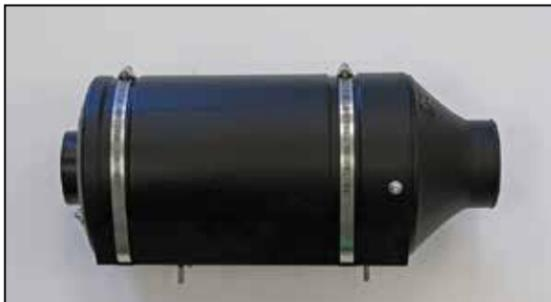
24. Secure the air filter housing to the bracket with the hose clamps as shown.
