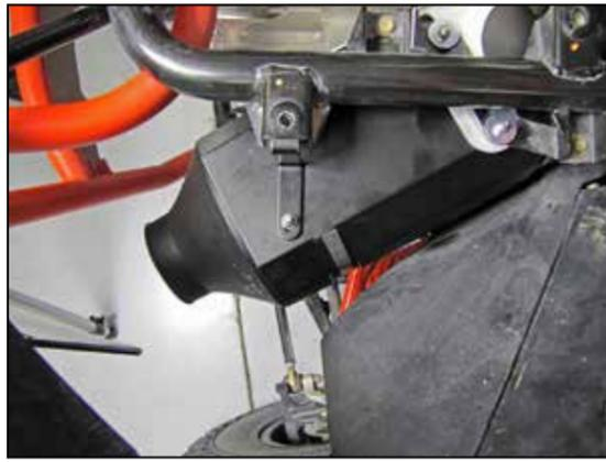
27. Install the provided mounting bracket (083110) as shown using the provided hardware.
