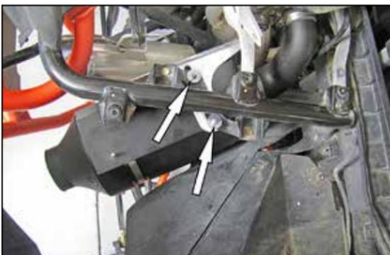
26. Install the factory heat shield onto the K&N® filter assembly then install the air filter housing assembly, engage the intake tube into the coupler hose and then align the front mounting studs to the factory air filter mounting position. Secure the K&N® housing to the front mounts with the hardware provided. Adjust the intake tube for best fit and then secure all the hose clamps.
