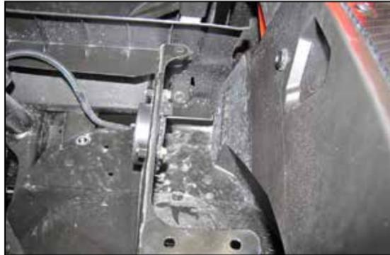
12. Remove the two bolts that secure the fresh air tube mount to the body and remove the mount.
