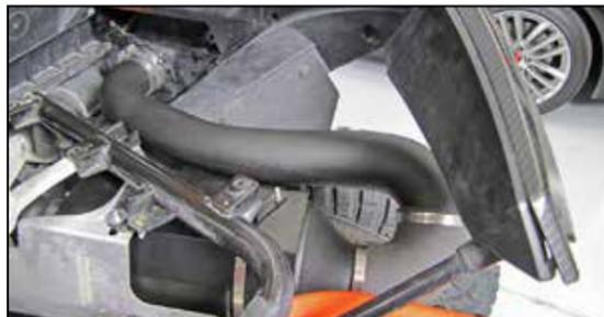
29. Install the K&N® fresh air intake tube assembly and 90° coupler hose (08502) to the fresh air tube mount and air filter housing, adjust for best fit and then secure with the provided hose clamps.
