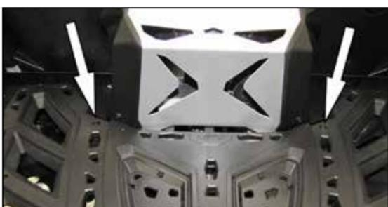
2. Remove the two bolts and nuts shown that secure the cargo tray to the frame.
