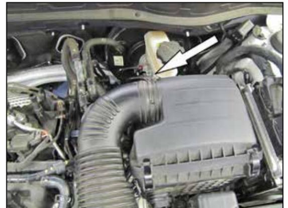
6. Loosen the hose clamp securing the factory intake tube to the air box and then remove the intake tube from the vehicle.
