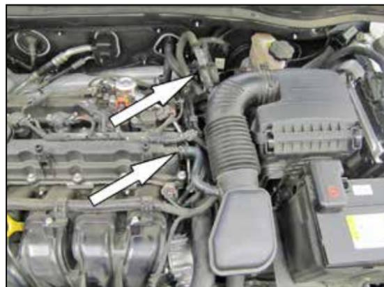
4. Disconnect the EVAP vent hose from intake tube and then disconnect the crank case vent hose from the valve cover.
