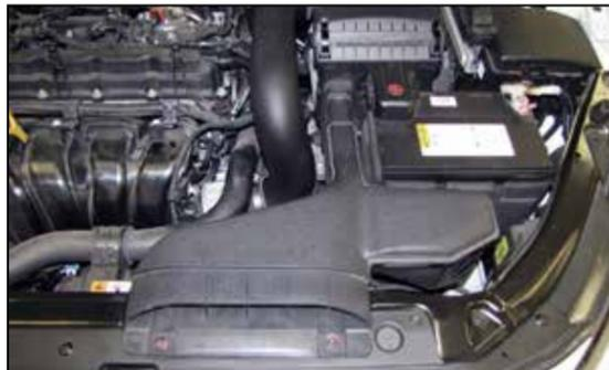
17. Reinstall the fresh air intake duct and secure with the factory bolts.
