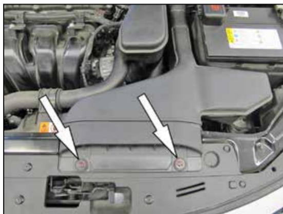
3. Remove the two bolts securing the fresh air intake duct to the core support and then remove the fresh air intake duct from the vehicle.
