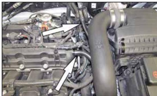
16. Connect the crank case vent line to the valve cover port and connect the EVAP vent line with the union and secure with the factory spring clamp.
