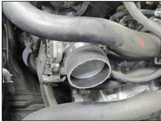
13. Install the provided coupling hose (08711) onto the throttle body and secure with the provided hose clamp.
