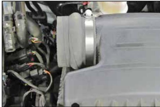
14. Install the provided hump hose (078121) onto the air box and secure with the provided hose clamp.
