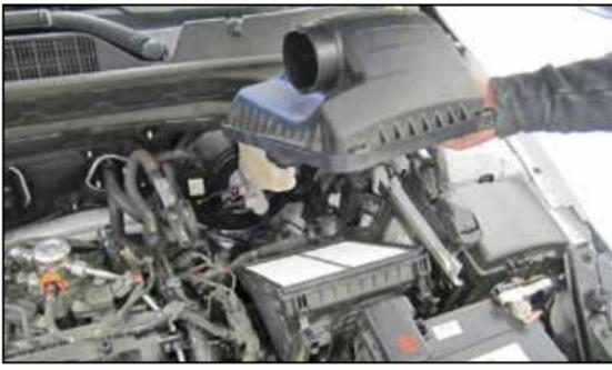
7. Release the four clips securing the upper air box; remove the upper air box and factory air filter.
