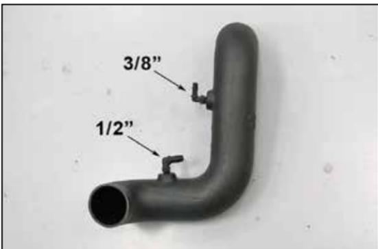
9. Install the two provided 3/8" and 1/2" 90° vent fittings into the K&N® intake tube as shown.
