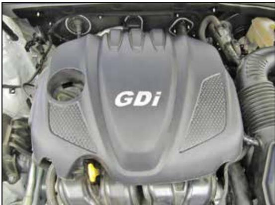
2. Lift up the engine cover and remove it from the engine.
