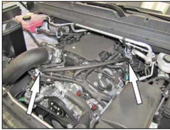
25. Install the crank case vent hose onto the fitting installed into the K&N® intake tube and then connect the hose mender into the fitting on the valve cover.
