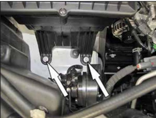
9. Remove the two nuts that secure the air filter housing to the inner fender and lift up the housing and remove it from the vehicle.
