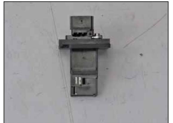
20. Install the factory mass air sensor into the K&N® adapter assembly and secure with the provided hardware.
