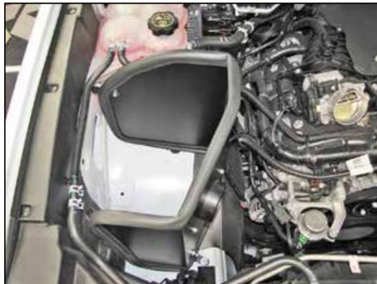
15. Install the heat shield so that the brackets set onto the coolant reservoir stud and the air filter housing mounting stud then secure the heat shield with the factory mounting nuts removed earlier.
