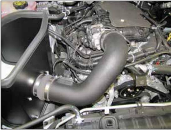
23. Install the K&N® intake tube into the hump coupler and then into the step coupler at the throttle body, adjust the tube for best fit and then secure with the provided hose clamps.
