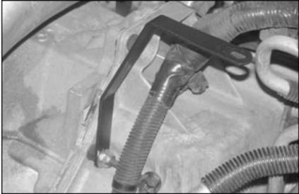
22. Install the K&N tube mounting bracket (07199) onto the stud exposed in step #21 and secure with the hardware provided.
