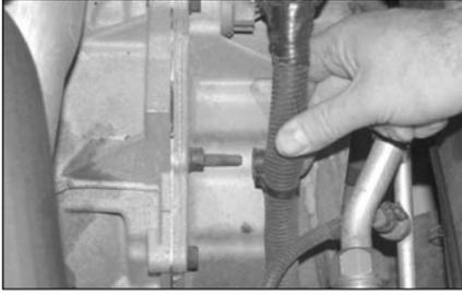
21. Remove the wiring harness retaining clip from stud protruding from the transmission case as shown.
