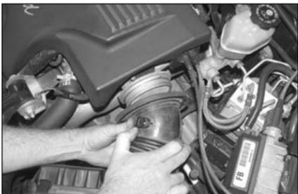
3. Pull firmly on the intake tube to separate the intake from the throttle body.
