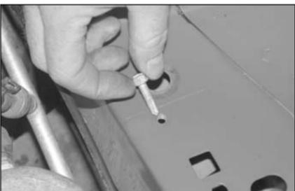
20. On vehicles that do not come equipped with a ground strap, use the 6mm self tapping bolt to thread the hole shown.
