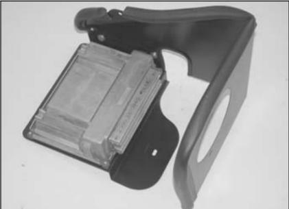
16. Install the engine processor onto the K&N heat shield and mounting bracket as shown.
