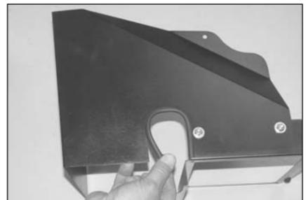
13. Install the small edge trim onto the heat shield assembly as shown.
