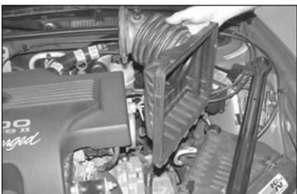
4. Release the two air box lid retaining clips, remove the air box lid and intake tube assembly as shown.
