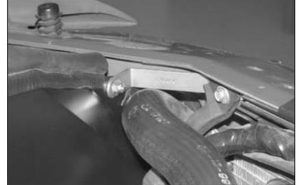
28. Reinstall the factory radiator bracket onto its original location with the K&N bracket (010056) so that the K&N bracket meets with the heat shield assembly and secure with the provided hardware.
