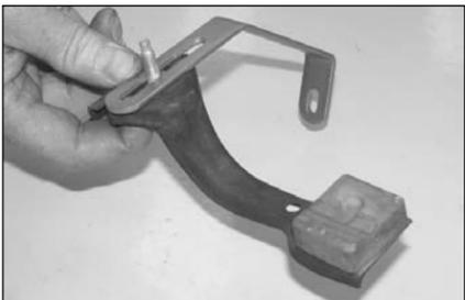
27. Place the K&N bracket (010056) behind the factory radiator bracket as shown.
