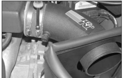
33. Install the K&N intake tube onto the throttle body, securing with the hose clamp provided, then secure the tube to the mounting bracket installed in step #22 with the provided 8mm bolt.
