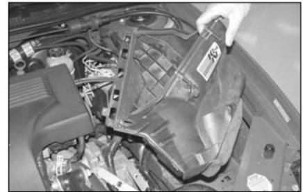
10. Pull firmly up on the engine processor housing to release it from the mounting tabs, then remove the housing from the vehicle.
