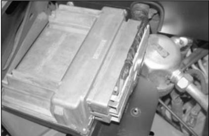
24. Reinstall the engine wiring harness connectors onto the engine processor and secure with mounting bolts.
