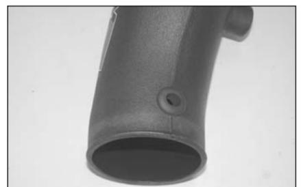
30. Install the provided grommet into the K&N intake tube as shown.
