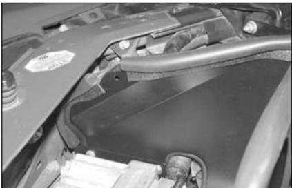
26. Remove the radiator mounting bolt and bracket shown.
