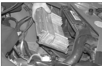
9. Remove the engine processor from its housing as shown.
