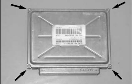
15. Remove the four processor cover plate bolts shown with a #27 Torx socket.
