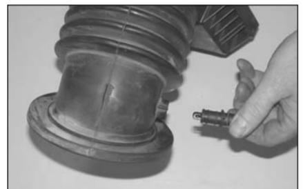
31. Remove the air temperature sensor from the factory intake tube.
