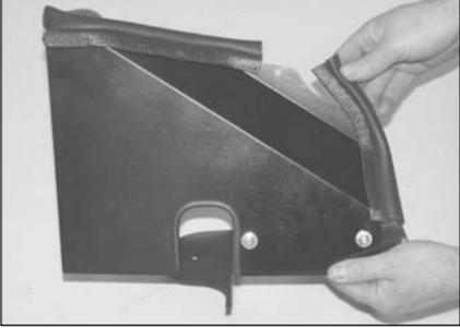
14. Install the large edge trim onto the heat shield as shown.
