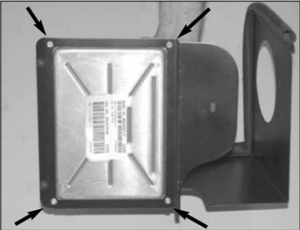
17. Install the four torx bolts remove in step #15 to mount the processor to the mounting bracket.
