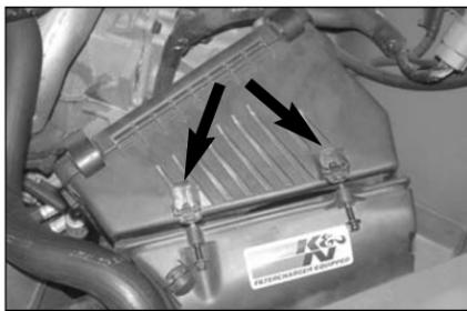
6. Loosen the two air filter housing mounting bolts shown.
