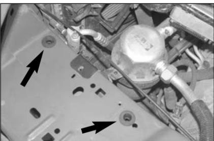
18. Remove the two air box mounting grommets shown by pulling them up out of the holes in the fender apron.
