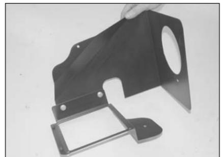
12. Assemble the heat shield to the processor mounting bracket using the provided hardware as shown.
