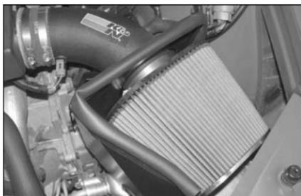
35. Install the K&N filter charger onto the intake tube and secure with the provided hose clamp.
