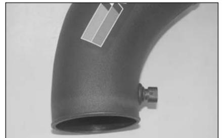
32. Install the air temperature sensor into the K&N intake tube as shown.
