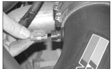
34. Reconnect the air temperature sensor electrical connection.
