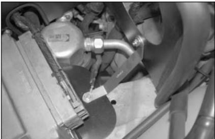
25. Install the heat shield mounting bracket (010057) using the provided hardware as shown.
