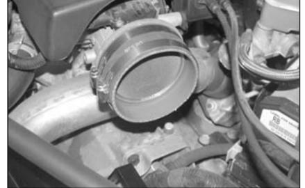
29. Install the silicone hose (08621) onto the throttle body and secure with the provided hardware as shown.
