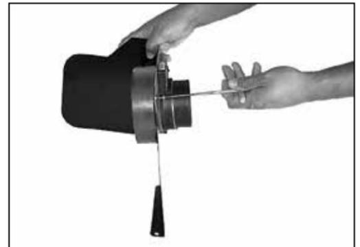
7. Assemble the mass air sensor, gaskets, heat shield and mass air adaptor with the provided hardware as shown.
