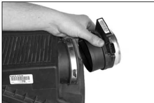
6. Loosen the hose clamp on the mass air sensor, then remove the mass air sensor.
