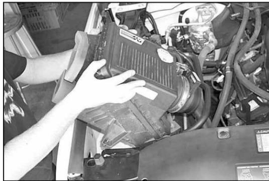
4. Pull firmly upward to release the air cleaner from its mounting grommets, then remove the air cleaner assembly.
