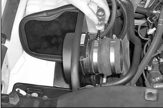
11. Install the silicone hump hose and hose clamps onto the mass air sensor as shown.
