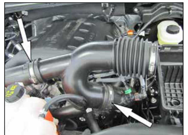
6. Loosen the hose clamps securing the intake tube to the two turbo inlet tubes and then remove the intake tube from the vehicle. NOTE: K&N Engineering, Inc., recommends that customers do not discard factory air intake.
