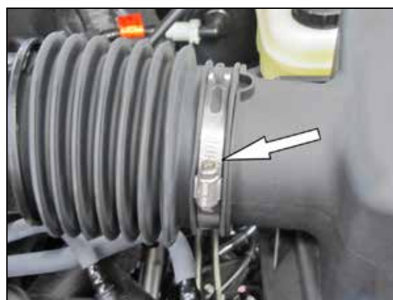
3. Loosen the hose clamp securing the factory intake tube to the air filter housing.
