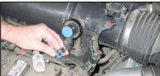
3. Disconnect the filter minder electrical connection.
