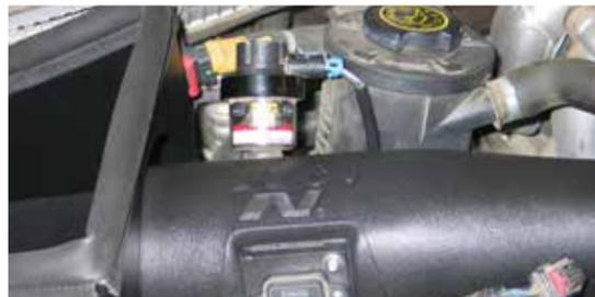
24. Attach the filter minder extension harness provided into the factory harness and then connect the open end to the filter minder.
