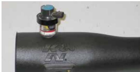
15. Install the filter minder and grommet into the K&N® intake tube as shown.
