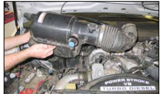
7. Lift up firmly on the complete air box assembly to dislodge it from the mounting grommets and then remove the complete air box and intake tube assembly from the vehicle.
