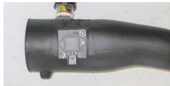
20. Install the mass air sensor assembly onto the K&N® intake tube as shown and secure with the provided hardware as shown.
