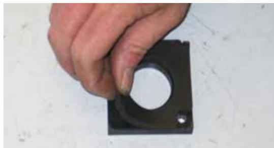
18. Install the provided gasket onto the K&N® mass air sensor adapter.
