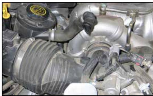
4. Clip the band clamp which secures the crank case breather hose to the intake tube. Then disconnect the breather hose and fitting from the intake tube as shown.
