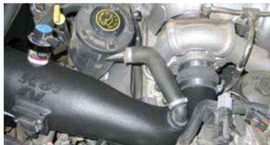
23. Insert the crank case vent fitting into the grommet in the K&N® intake tube.
