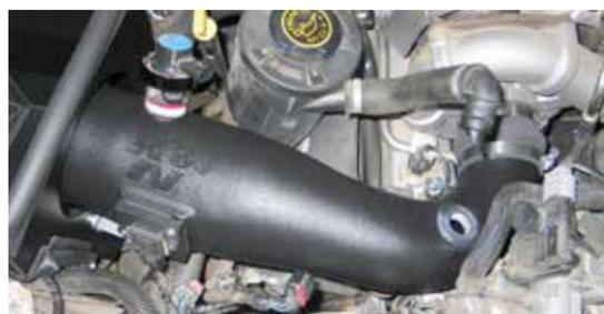
22. Install the K&N® intake tube assembly into the heat shield and slide the silicone hose onto the turbo inlet. Secure the intake tube to the mounting bracket on the heat shield with the provided hardware and then position the silicone hose onto the turbo and secure with the hose clamps.
