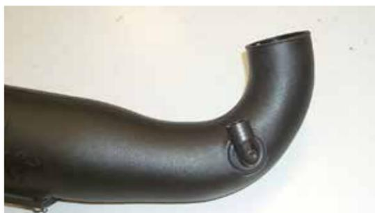
16a. On models that have the crank case vent fitting attached to the stock intake tube, install the supplied 90° vent fitting into the grommet as shown.
