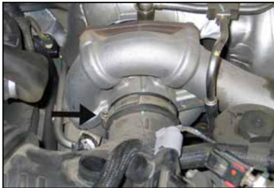
5. Loosen the hose clamp which secures the intake tube to the turbo inlet.
