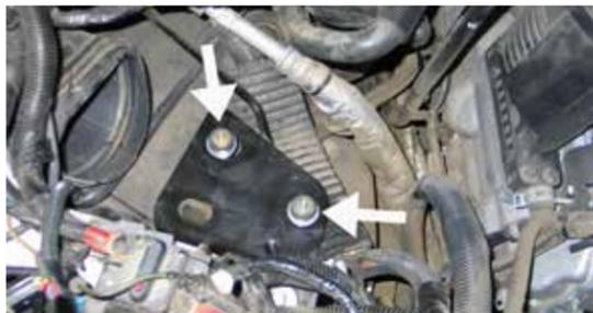
11. Install the provided rubber mounted studs onto the heat shield mounting tray using the provided hardware.
