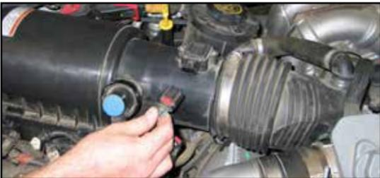
2. Disconnect the mass air sensor electrical connection and unclip the wiring harness from the air box as shown.
