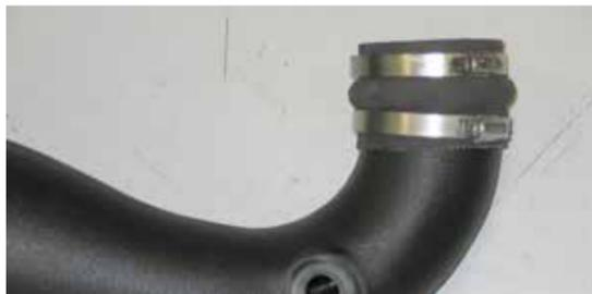
21. Install the provided silicone (087121) hose onto the K&N® intake tube with the hose clamps provided as shown.
