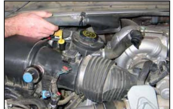
6. Unhook the warm air inlet tube from the fire wall as shown.
