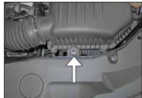
6. Remove the bolt that secures the air filter housing to the core support.
