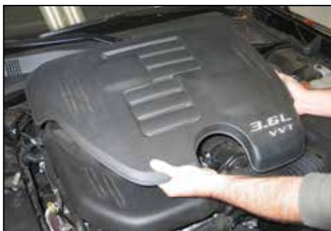
2. Lift up and remove the engine cover.
