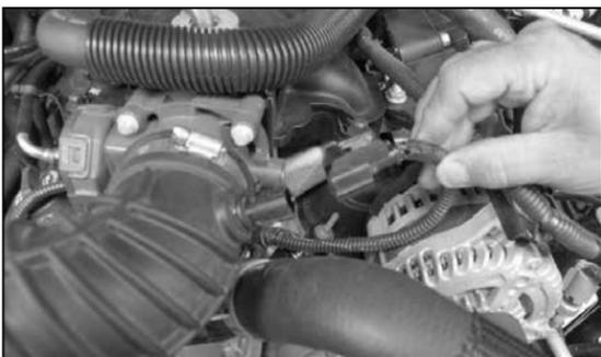
2. Release the locking tab on the air temperature sensor electrical connector and then disconnect the connection.
