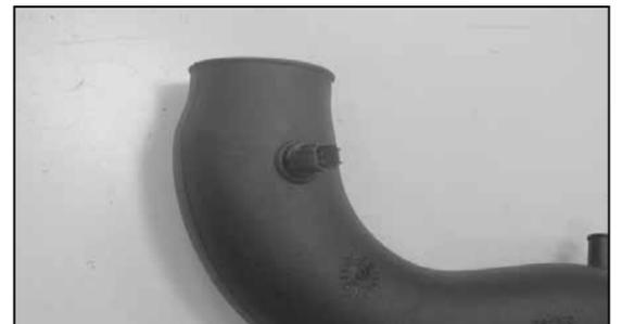
8. Install the air temperature sensor into the grommet installed into the intake tube in step #6.
