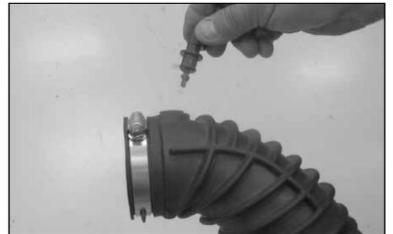
7. Remove the air temperature sensor from the stock intake tube as shown.
