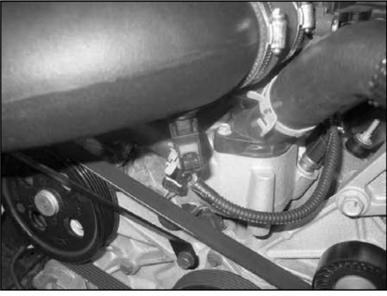
25. Reconnect the air temperature sensor electrical connection.
