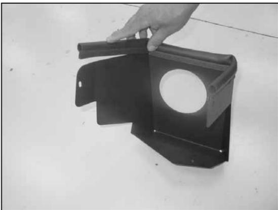
14. Install the supplied edge trim onto the heat shield as shown.
