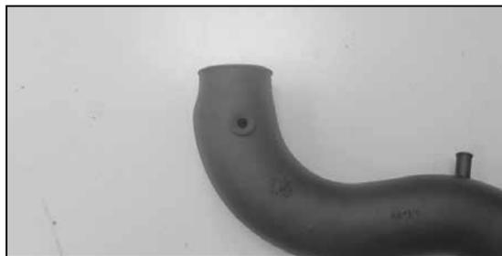
6. Install the supplied grommet into the hole in the intake tube as shown.
