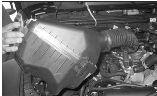
5. Lift up the airbox assembly to dislodge it from the mounting grommets and then remove the complete assembly from the vehicle.
