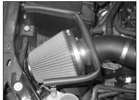
24. Install the K&N® air filter assembly on the intake tube and secure with the provided hose clamp as shown.
