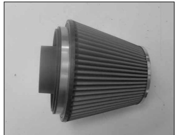
22. Install the air filter adapter into the K&N® air filter and secure with provided hose clamp.
