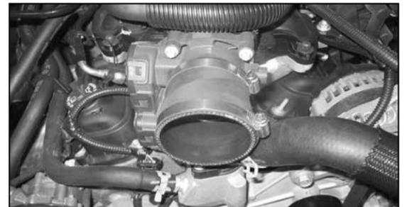
9. Install the supplied silicone hose onto the throttle body and secure with the supplied hose clamp.
