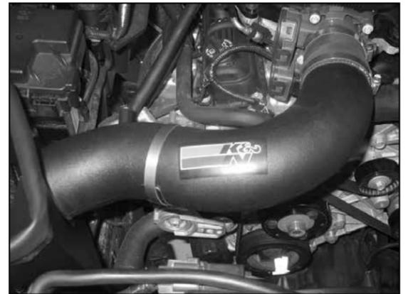
20. Insert the intake tube into the silicone hose at the throttle body and align with the mounting bracket installed in step #12 and then secure with the hose clamps provided.
