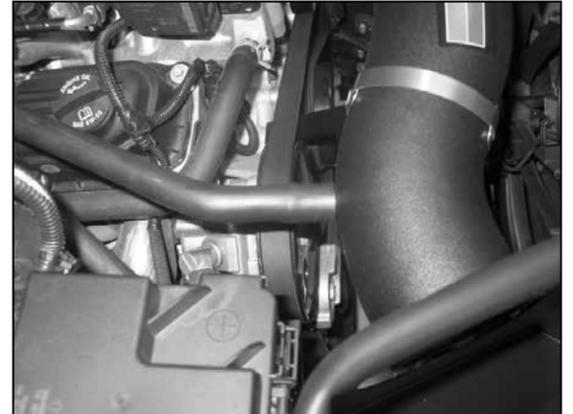
21. Connect the crankcase vent hose to the intake tube.
