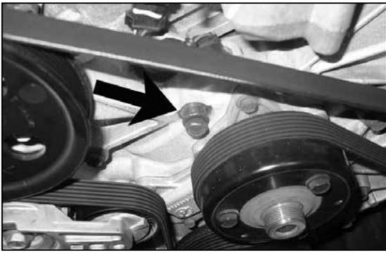
10. Remove the front engine bolt shown.
