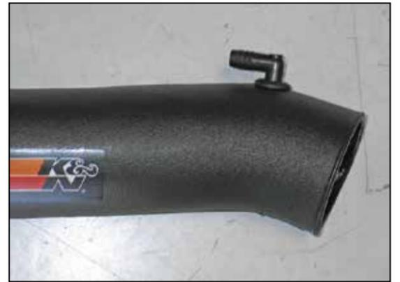
16d. On SRT 8; 6.1L equipped vehicles, install the provided 90° hose mender as shown.
