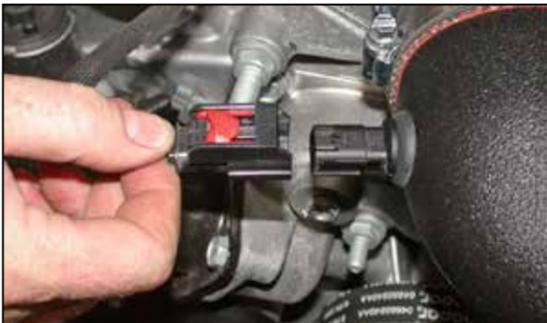
23. Reconnect the air temperature sensor electrical connection as shown.
