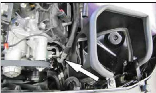
11a. Due to vehicle manufacturing tolerances, the A/C lines on some vehicles may need to be repositioned slightly so that they do not contact the heat shield. To adjust, grab the A/C line on the aluminum section and carefully apply pressure in the desired direction until clearance is obtained.
