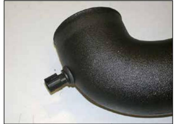
17. Install the factory air temperature sensor into the grommet installed in step #16.
