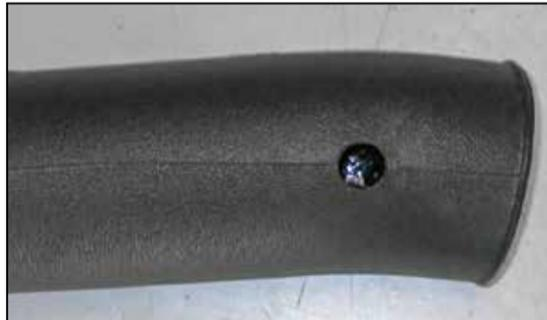
16b. Drill out the hole in the intake tube to 0.75".
