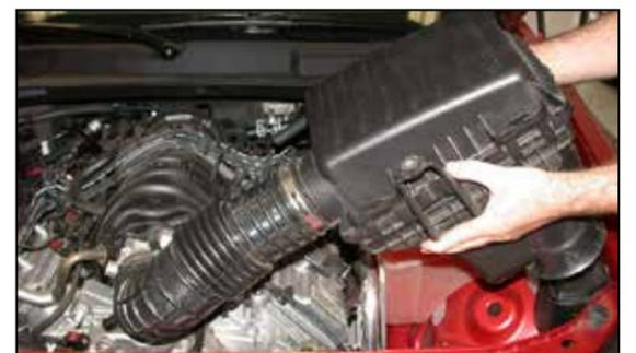
7. Lift the complete intake and air filter assembly to remove it from the vehicle.
