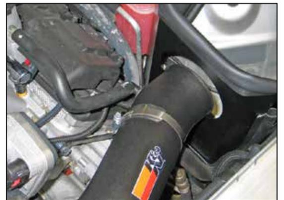
19a. On SRT 8; 6.1L equipped vehicles, connect the factory crank case vent hose onto the 90° fitting installed into the K&N® intake tube (in step #16c).
