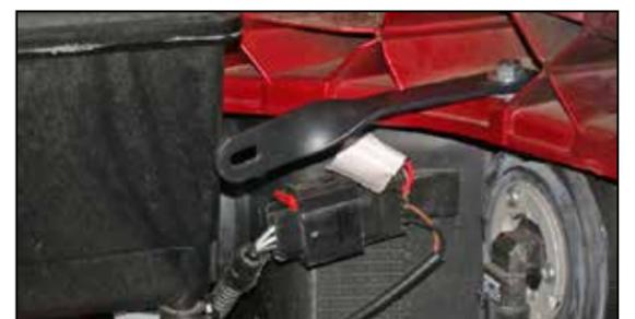
8. Install the twist bracket (070772) onto the core support using the hardware provided through the existing hole as shown.
