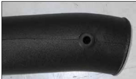
16c. On SRT 8; 6.1L equipped vehicles, install the provided grommet into the 0.75" ID hole as shown.
