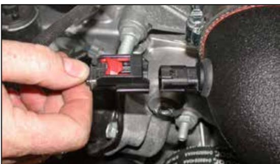
3. Unlock the red locking tab on the air temperature sensor electrical connection, then depress the locking lever and pull apart the temperature sensor electrical connection.
