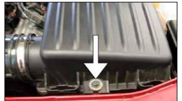
6. Loosen and remove the air box mounting bolt as shown.
