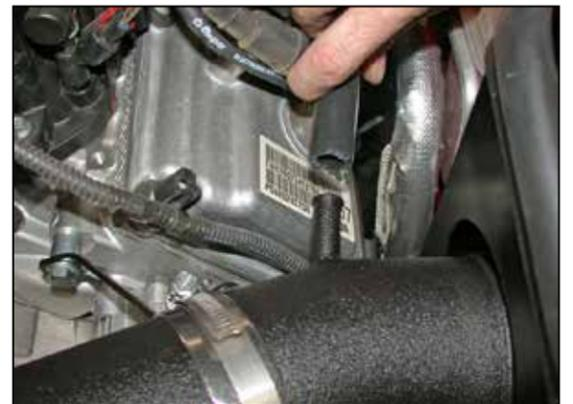
19. Install the provided crank case vent hose onto the vent port on the valve cover then install the vent hose onto the K&N® intake tube.
