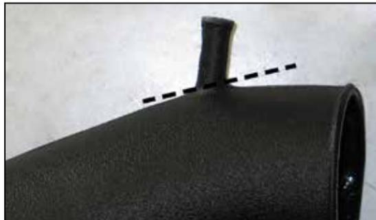
16a. On SRT 8; 6.1L vehicles, cut the vent off of the K&N® intake tube as shown.
