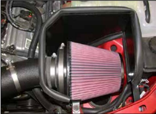
22. Install the air filter assembly onto the K&N® intake tube and secure with the provided hose clamp as shown.
