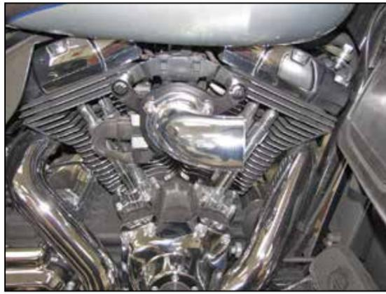
10. Install the two remaining O-Rings and K&N® breather bolts into the tube adapter. Tighten all of the hardware at this time.
