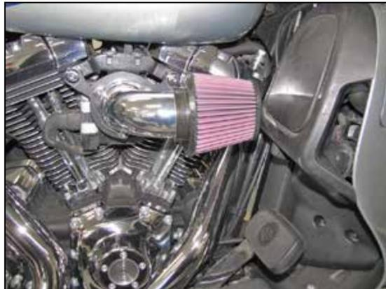
11. Install the K&N® air filter and secure with the provided hose clamp.
