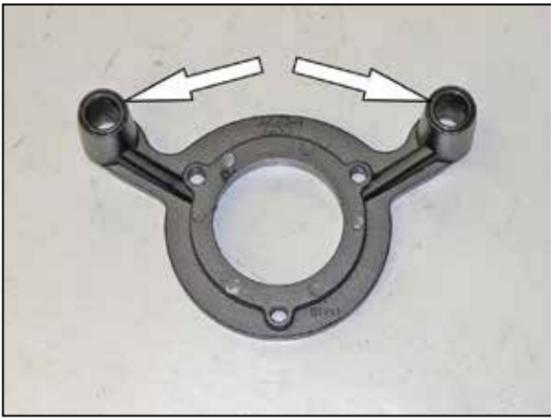
7. Install two of the provided O-Rings into the engine side of the K&N® intake tube adapter.
