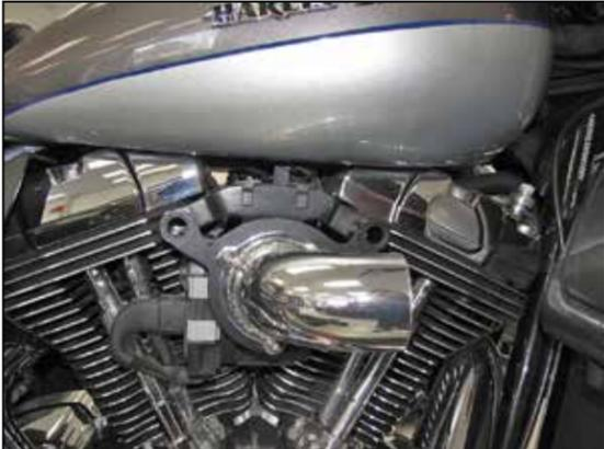
9. Apply one drop of the provided thread locker onto the tube mounting bolts. Install the complete tube and adapter assembly onto the throttle body and secure with the tube mounting bolts.
