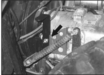
20. Install the lower air box bracket (#09496) onto the shifter cable bracket at the left side of the transmission as shown.
