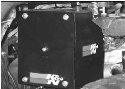
32. Install the K&N® air box cover, aligning the ¼" bolt in the filter with the center hole in the cover on the K&N® air box. Secure with the provided hardware as shown.
