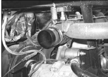
21. Install the K&N® intake tube into the factory rubber manifold and secure with the factory clamp removed in step #18 as shown.
