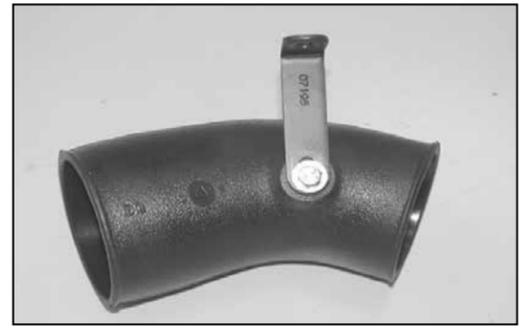
18. Install the tube mounting bracket (07195) onto the intake tube with the provided hardware.
