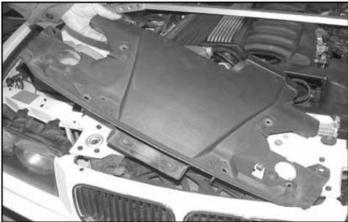
9. Lift the radiator cover from the rear to unhook from the alternator fresh air supply. Remove the cover from the vehicle.
