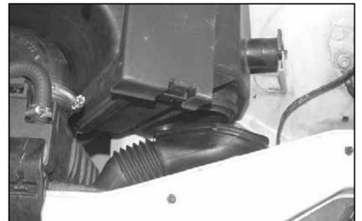
5. Using a flat blade screwdriver, dislodge the fresh air duct from the air box as shown.
