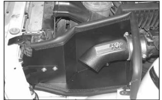
19. Install the intake onto the mass air sensor, then secure with the provided hose clamp and secure the tube mounting bracket to the heat shield with the provided hardware.
