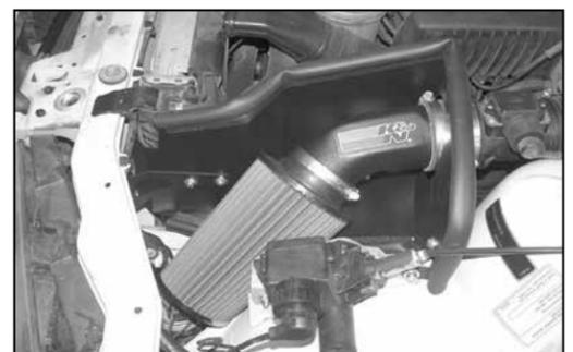
22. Install the K&N® air filter and secure with the provided hose clamp.
