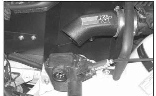
20. Re-install the speed control removed in step #3 to the mounting brackets with the provided hardware as shown.
